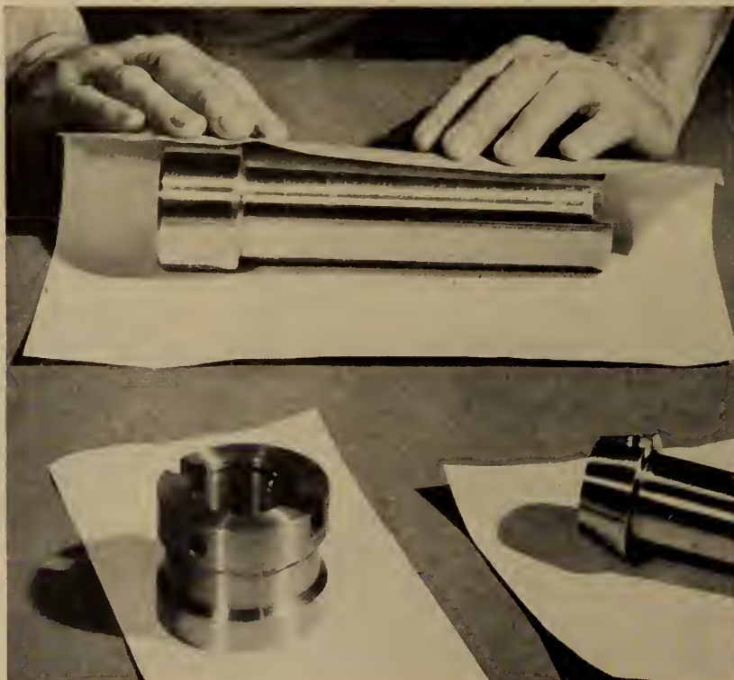
Fig. 2. Packing pump parts in wrappers impregnated with vapor phase inhibitors.
