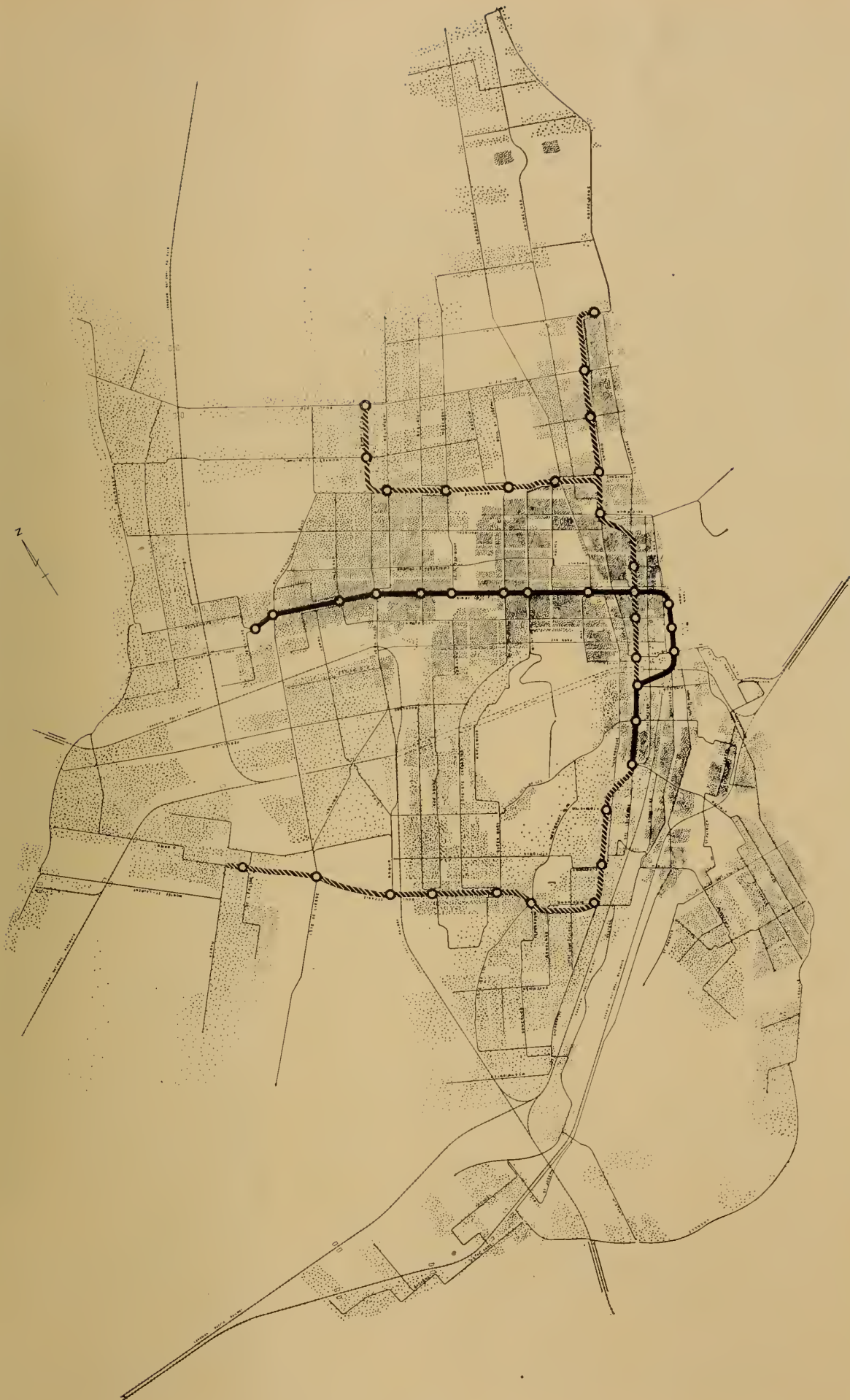
Comprehensive Plan of Proposed Subway System, with Possible Pattern of Surface Routes. : : Forecast of population distribution, 1971. — Initial subway project. - - - - Future subway. ○ Subway stations. — Passenger railway lines. + + + + Surface transit routes.
