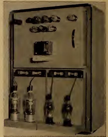
Fig. 3. Adjustable speed control panel: "brain" unit at top; motor armature rectifier testers at bottom left; motor field rectifiers at bottom right.
