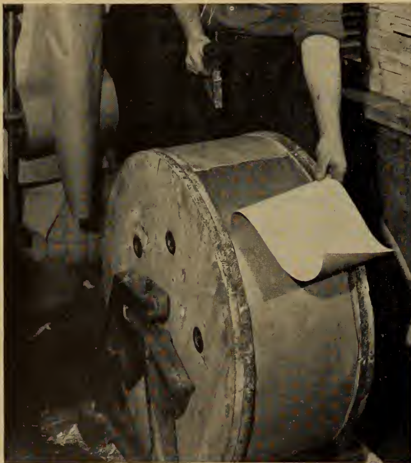
Fig. 1. Wire is cleanly and quickly packed with paper impregnated with the volatile inhibitors.
