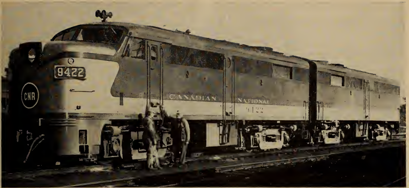
Fig. 1. Diesel road freight locomotive, 3,200 hp.
