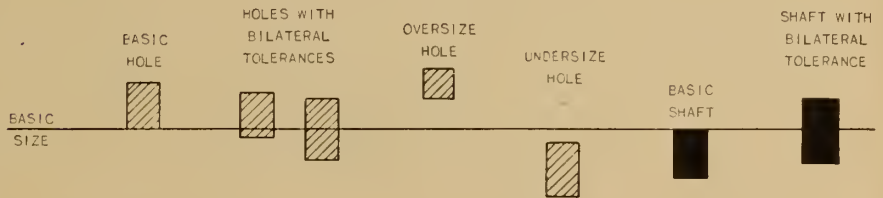
Fig. 3. Tolerance zones for various holes and shafts.
