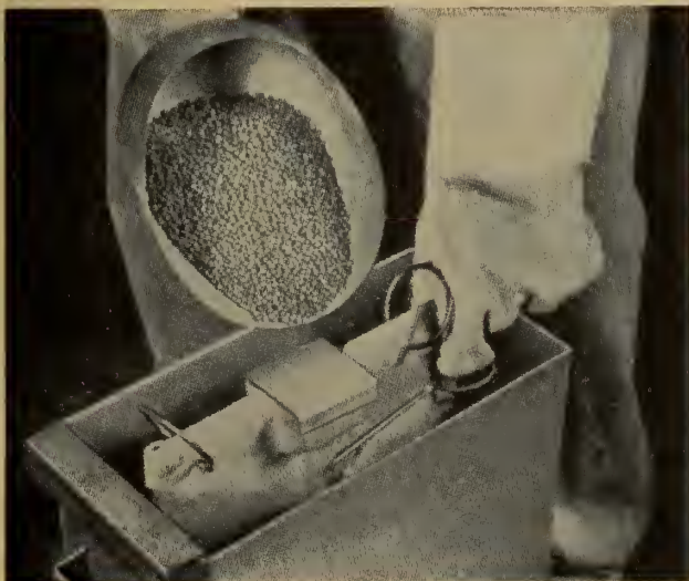
Fig. 3. Mold backed up for pouring.
