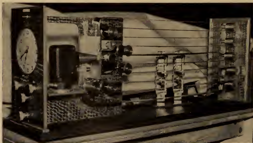
Fig. 6. Automatic train dispatcher.
