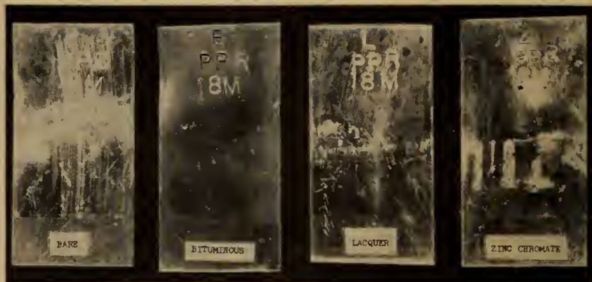
Fig. 7. Alcan 3S sheet specimens removed from a portland plaster (stucco) wall section exposed outdoors for 18 months. Notice only slight superficial attack confined to the 3/4" band of contact with the stucco.
