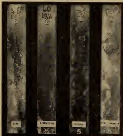
Fig. 6. 50S-A33 specimens from the dry lime brick mortar pier after 18 months. Note the effectiveness of the bituminous paint coating.
