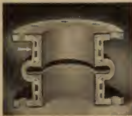
Sectional view shows sturdy construction of single orifice joint. Arrow points to one of steel reinforcing rings
