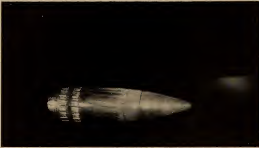
Fig. 3. Microflash photograph of a 6-pounder shot in flight at 2,800 ft. per second.
