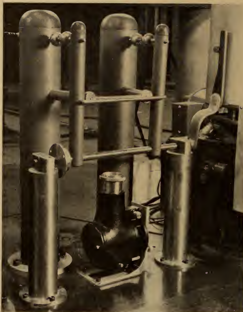
Fig. 5. Tripping mechanism: pin in main moving column at top right.
