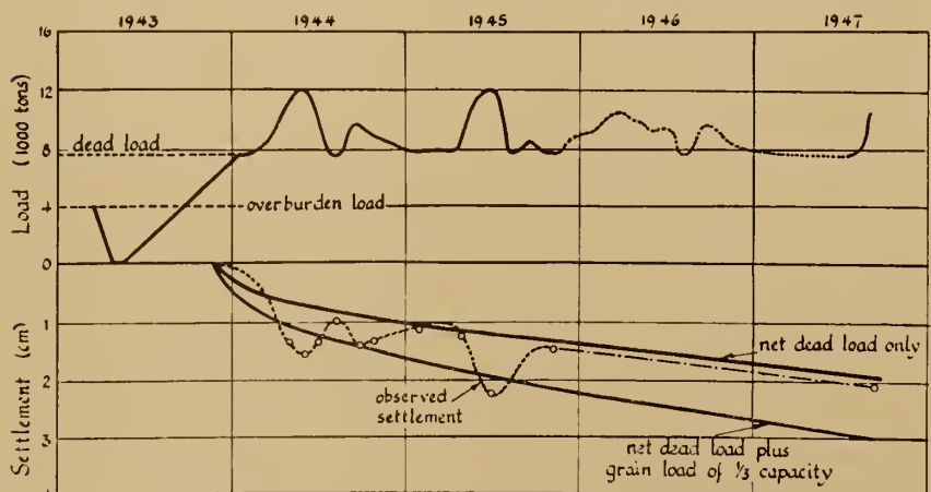
Fig. 3. Comparison of observed and estimated settlement of grain elevator on clay with variable foundation load.
