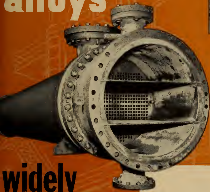
This 33-inch vapor condenser built for McColl-Frontenac's Montreal refinery is lined with 20% Monel-clad to resist corrosion from hot oil vapors. Cooling tubes inside are 70-30 cupro-nickel.
