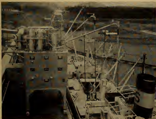
Fig. 118. Pneumatic alumina unloading plant.
