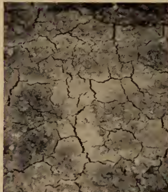
Effect of Drying Shrinkage is Dramatically Illustrated in this Clay Specimen.
