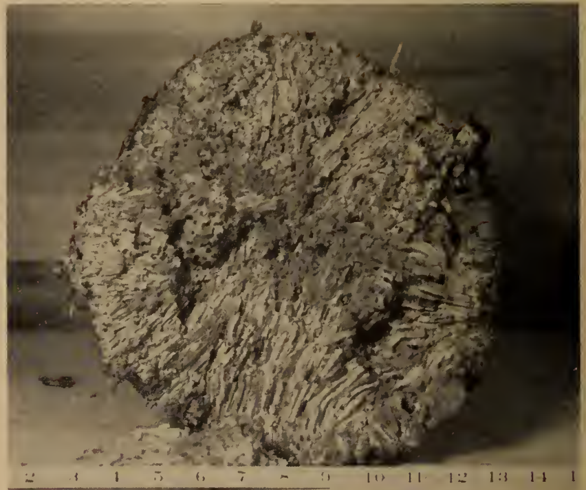
Fig. 75. What Teredo Navalis did to a pile in six months.
