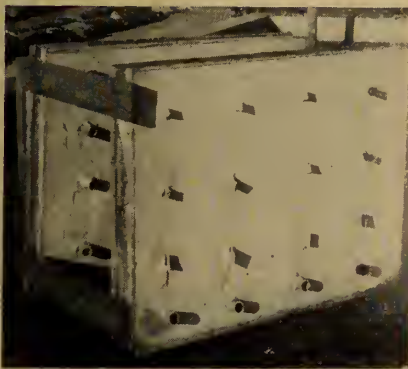
Fig. 1. Alcan 3S, 50S and 65S specimens exposed on the roof of the laboratory embedded in (a) concrete blocks (b) two types of mortar in "dummy brick walls" (c) plaster on "mocked-up" wall sections.
