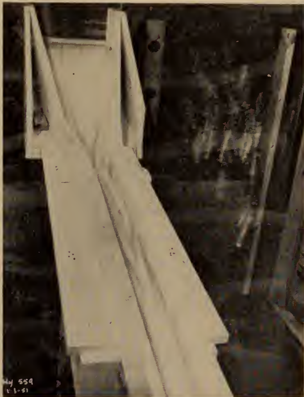
Fig. 9. Log chute model test in the hydraulic laboratory of the National Research Council.
