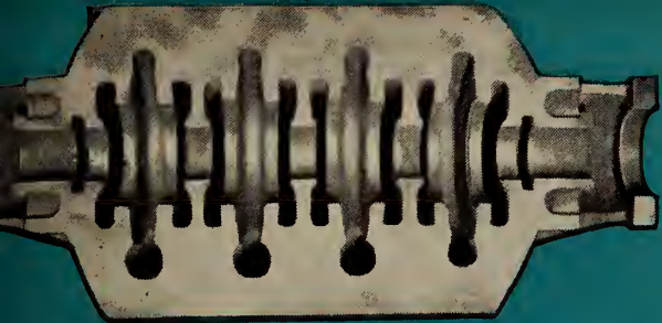
Interior view showing lower half of pump made of high nickel alloy by Shawinigan Chemicals Limited, Stainless Steel and Alloys Division, Shawinigan Falls, P.Q.
