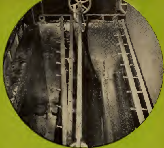
Chromium-nickel stainless steel head box on a Fourdrinier machine in the plant of Provincial Paper Limited, Thorold, Ont.
