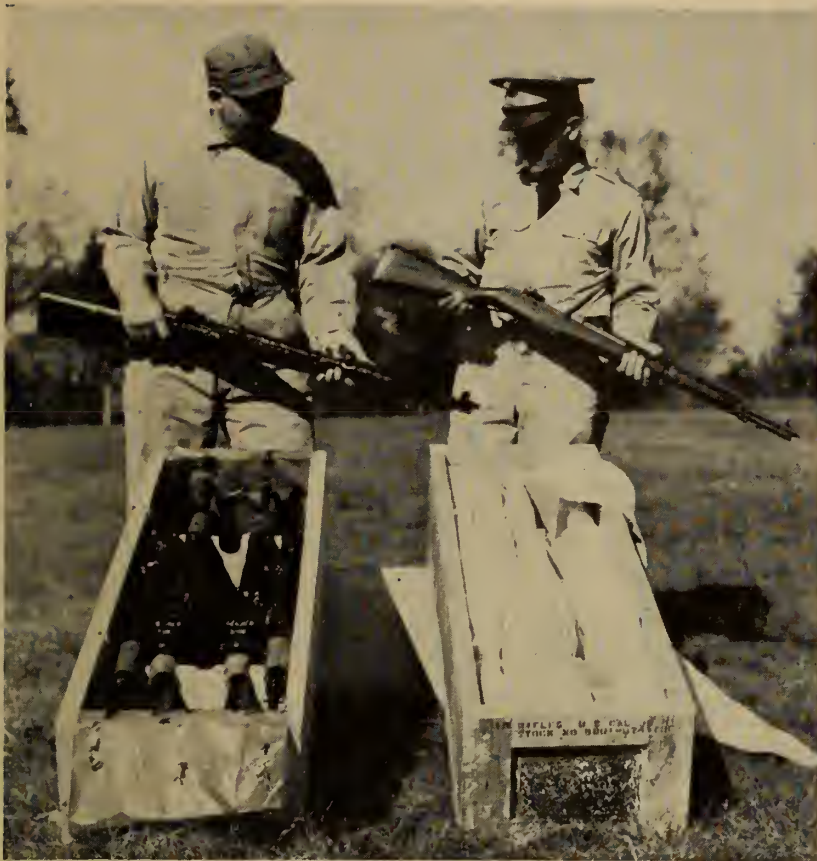
Fig. 3. The rifle packed in paper impregnated with vapor phase inhibitor (right), is clean and ready for immediate use, while the rifle packed in grease must be cleaned before it is ready for firing.
