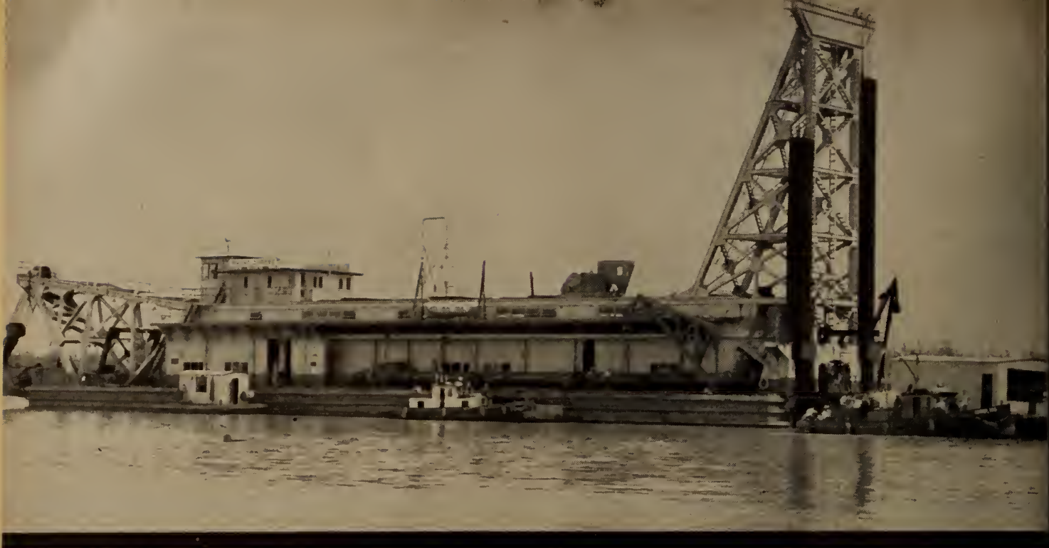
280 feet from stem to stern, the 2500-ton "Hydro-Quebec" is shown in a rare idle moment. Over a period of several years of dredging, the 26-ton cutter will chew out an estimated 50 million tons from the 3,300 feet wide and 15 mile long canal, deepening the whole canal to 35 feet. Submarine cable supplies 13,800 volts for the vessel's electrical equipment.
