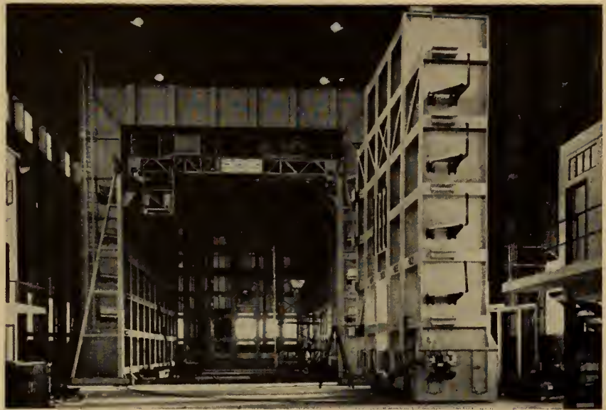
Fig. 9. Testing frame for full-scale structural components.
