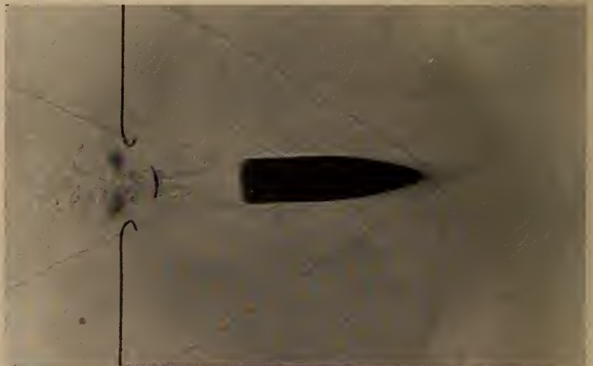
Fig. 4. Spark shadowgraph of a service rifle bullet in flight.
