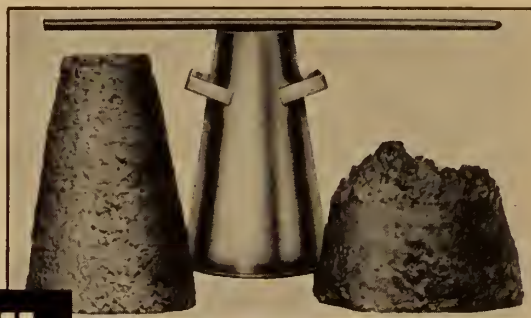
Pozzolith Produces Greater Slump with Some Amount of Water
