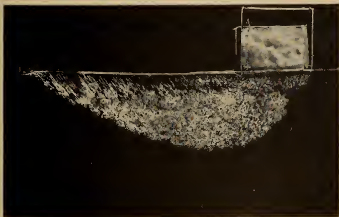
Fig. 1. Failure zone below rectangular footing on surface of dense sand.
