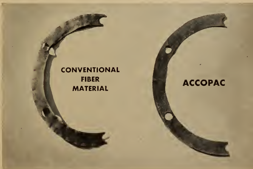
NEVER DRIES OUT. These two fiber sheet gaskets were used for 6 months in a gear pump circulating hot hydraulic oil. The conventional gasket lost its glycerine plasticizer, dried out, shrunk, hardened — and leaked badly. The Accopac gasket remained virtually unaffected as shown in the above photo.
