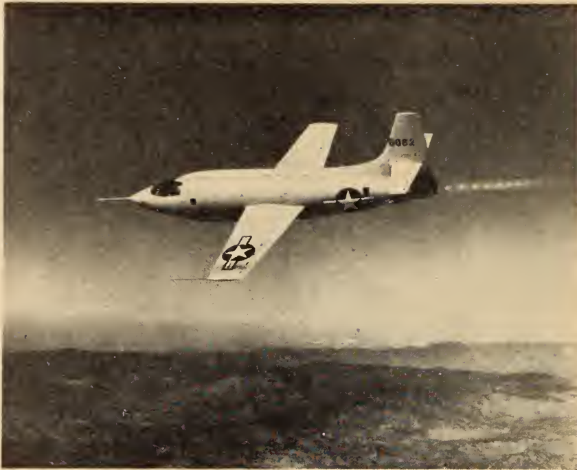
Fig. 4. The X-1 at high altitude cruising under power. Note shock-wave patten in the exhaust jet.
