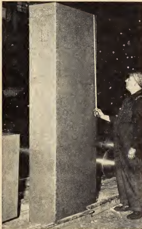
This illustration shows larger size Die Blocks made for the forging of aircraft parts.
