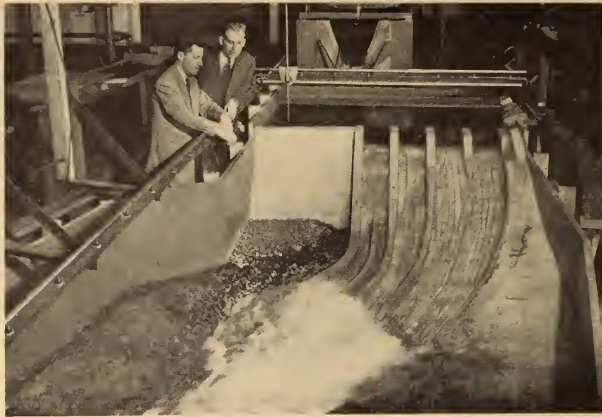
Fig. 4. The sluiceway design was developed with the help of model studies in the hydraulics laboratory at Ecole Polytechnique, Montreal. Shown here during testing are Prof. R. Boucher and J. A. Thomas, hydraulic engineer, Shawinigan Engineering Co., Ltd.
