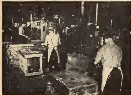
Here, two sheets of Anaconda Manganese Brass are being welded to form a refrigerator evaporator.
