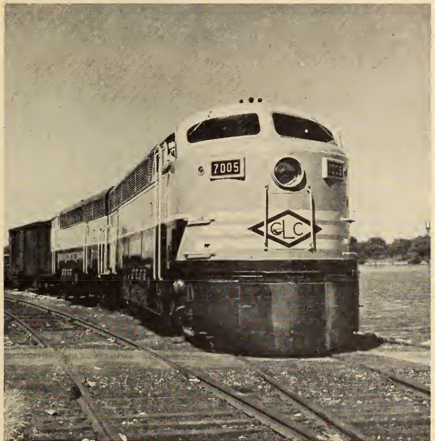
The "City of Kingston", first of the Consolidation line of diesel-electric road locomotives to be produced in Canada by the Canadian Locomotive Company, Kingston. Prototype of a line of Consolidation Locomotives, this first model is a road freight locomotive, capable of hauling heavy freight trains at 65 m.p.h. The passenger version of this locomotive will haul a full train at 110 miles an hour.
