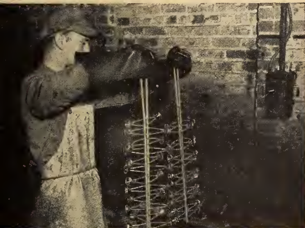
In this tank coupling nuts are immersed for copper, nickel and usually chromium plating.
