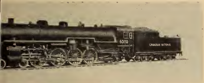
Number 6000, historic Mountain type engine built by C.L.C. in the early '20's.
