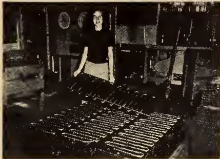
Copper tube is shown assembled into position ready for brazing for refrigerator condenser plates.
