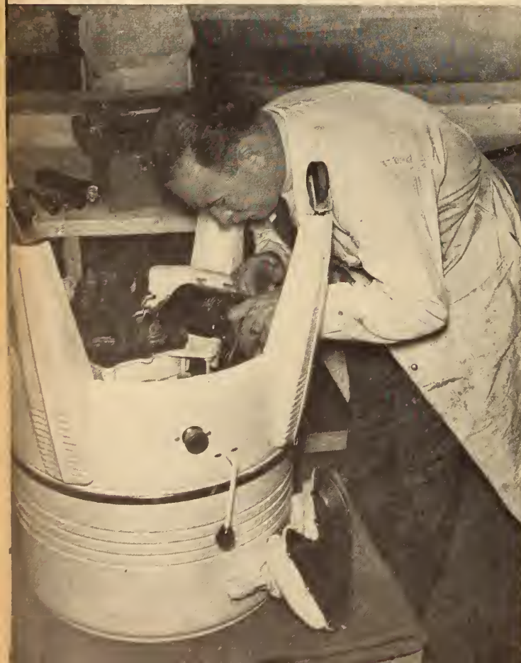
Fig. 7. Technician is shown converting washing machine motor for 60-cycle operation. More than 550,000 of these appliances must be changed over during conversion.
