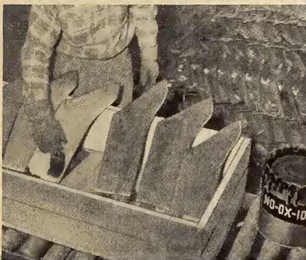
Applying NO-OX-ID rust preventive to plowshares by means of brushing.
