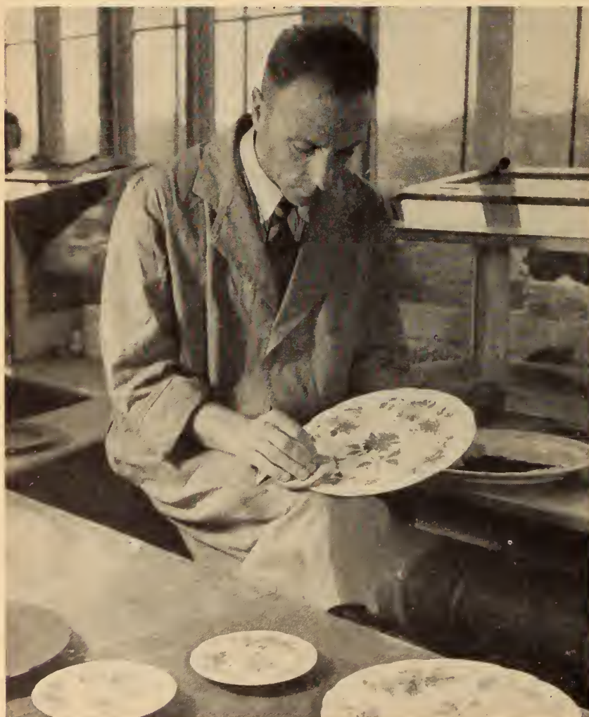
Fig. 3. The tradesman in this photograph is a "groundlayer". He coats the china with oil "size" and the color is dusted on to the oil. The ware is then fired.
