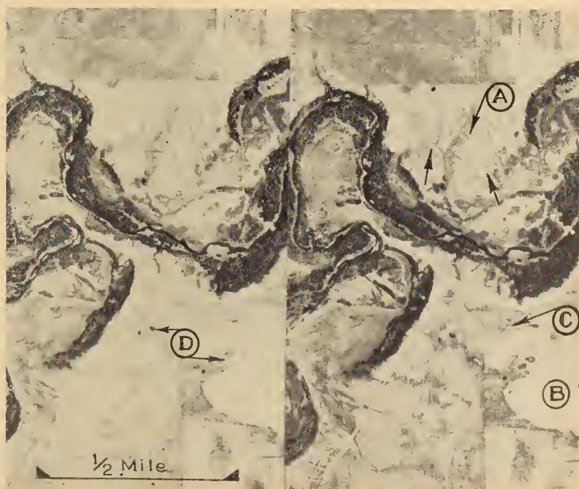
Fig. 4. A stereopair of a Valley Section and Adjacent Upland Soil Conditions. Small, closely spaced, notch-like gullies at A indicate deep, clean sands and gravels. The solid white area, B, indicates local soil drifting. Surface soils on the upland are sandy (inferred from light colour tones and the ease with which soils drift). The sandy soils are only a thin mantle, and overly relatively impervious soil materials (inferred from water in small depressions, D). C points to small, eroded, "burn-out pits," associated with alkali conditions. Note, also, the many changes in valley side slopes shown in this stereopair.
