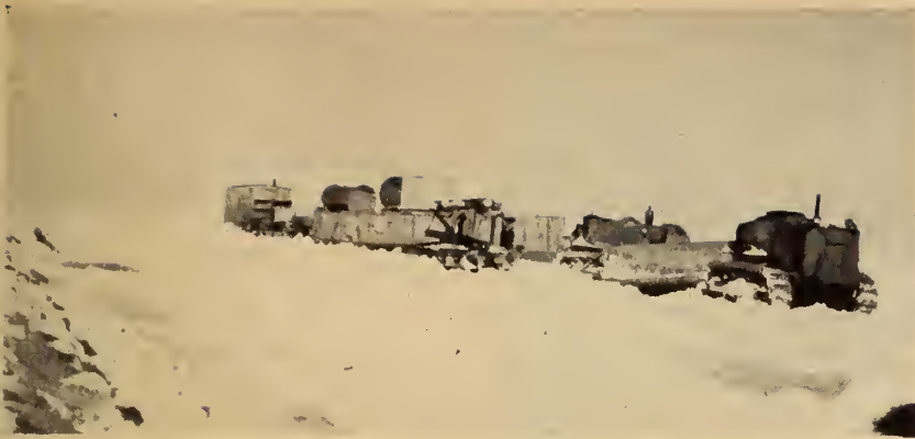
Fig. 2. Tractor train on Great Slave Lake, carrying parts of 6000-kva. generator. Note front tractor required to help start the train moving and also the caboose in which the crew eat and sleep.
