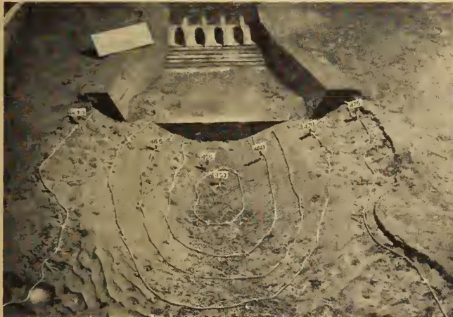
Fig. 1. (upper left). Model of old-fashioned 900-cusec drop. Fig. 2. (upper right). Drop of Fig. 1., improved by standard spreading floor; downstream floor inadequate.
