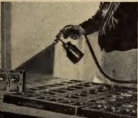
Typical spray gun application of NO-OX-ID rust preventive on engine head castings.
