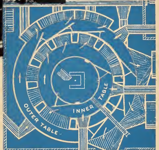
Construction view and diagram showing rotary table unit. This is the hub of a conveyor system between the log haulup, barkers, chippers and wood yard of a pulp mill.
