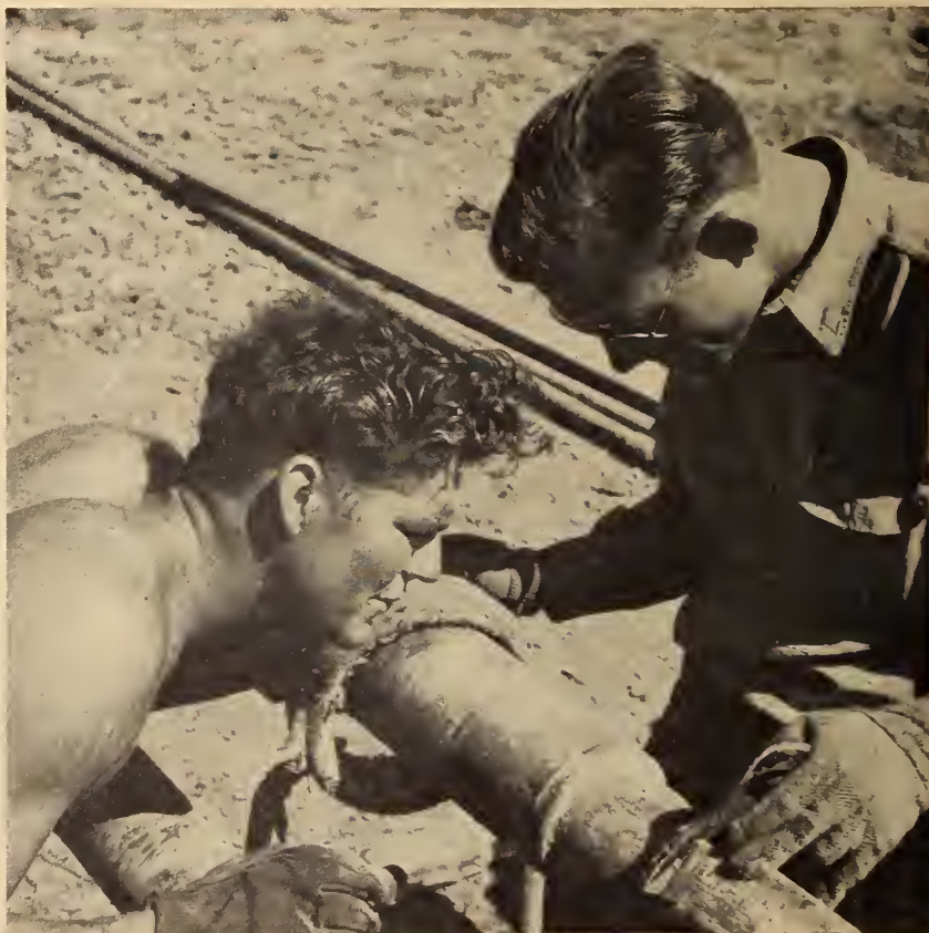
Fig. 2. Flaws in drill pipe may lead to breakage during drilling operations which might result in a costly "fishing" job. These men are using a magnetic coil to magnetize a piece of drill pipe. Powdered iron sprinkled on the magnetized pipe will reveal the presence of hidden cracks or other weaknesses.
