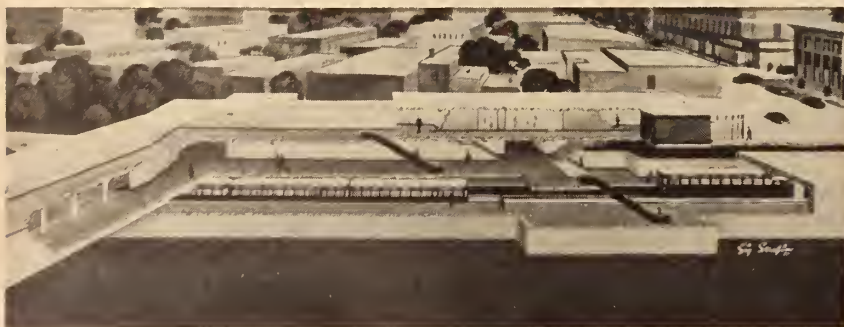
Fig. 6. St. Clair Station. At this station a cross-town surface street car line will load and unload passengers at each track. The street car platforms are connected with the subway platforms by escalators and stairs.
