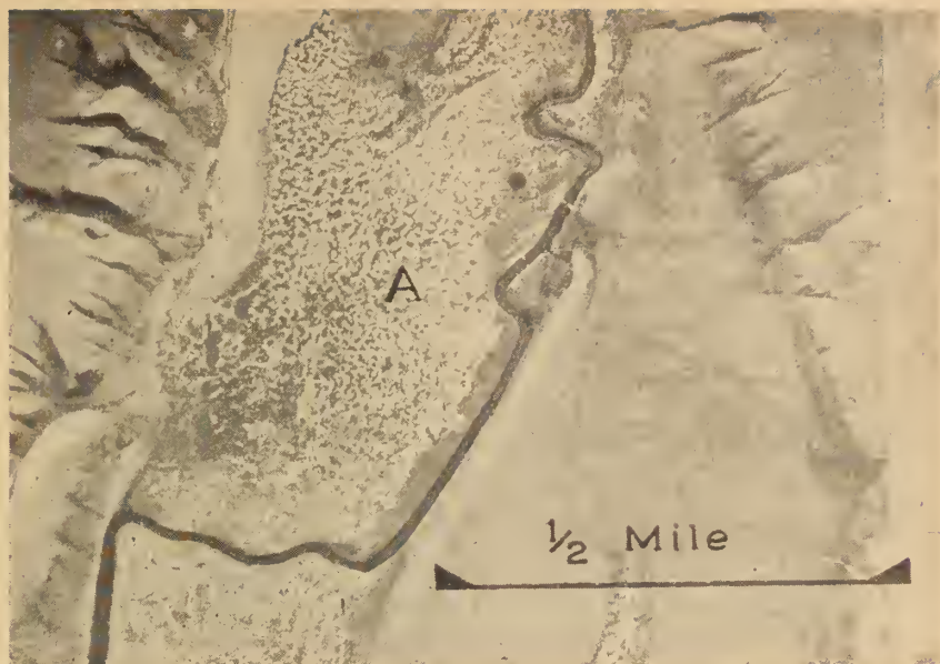
Fig. 7. Alkali-salt pattern. The speckled light and dark pattern at A indicates a high concentration of alkali-salts in the surface soils. Many variations of this pattern are readily identifiable (Fig. 4). Right-angle bends in the river suggest a fracture or jointed system in the bed rock that is near ground surface.
