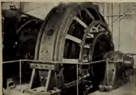
1350 hp mine hoist d-c motor.
