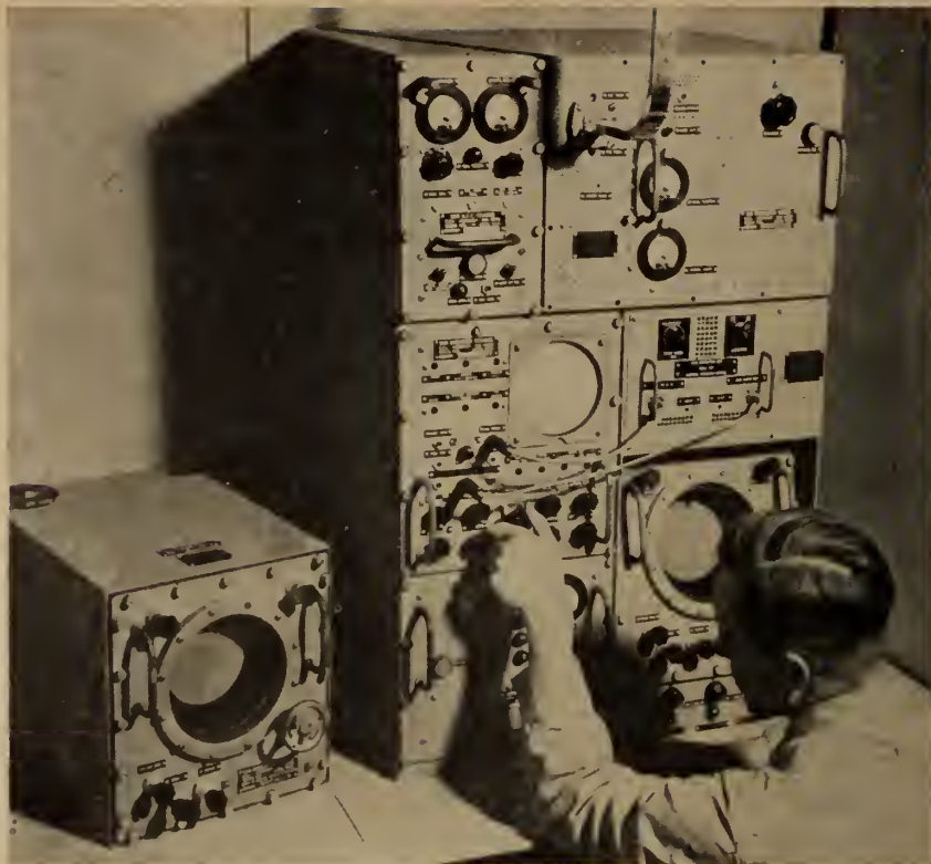
Fig. 6. Type 268 marine radar set developed for naval service.
