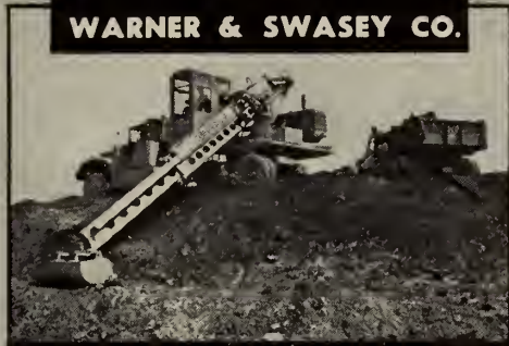
Fast, telescoping action of boom makes digging and loading one continuous operation... loading out dirt in record breaking time.
