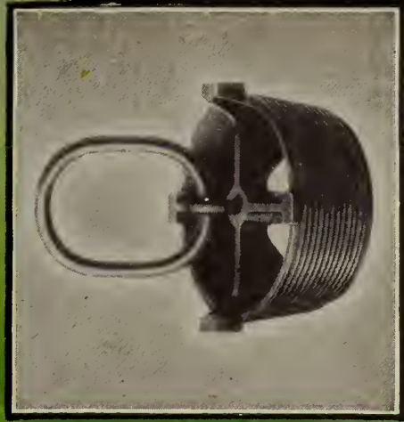
Lifting plug for 20" dia. electrodes—Weights 40 lbs. Old Type—97 lbs.
