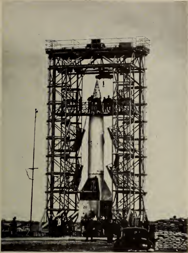
Fig. 5. Final instruments are placed in V-2 by technicians prior to flight into ionosphere.
