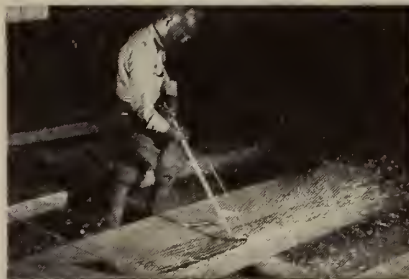
The descaling blowpipe, equipped with the OXWELD starting-rod feed, has reduced conditioning costs more than 50 per cent.
