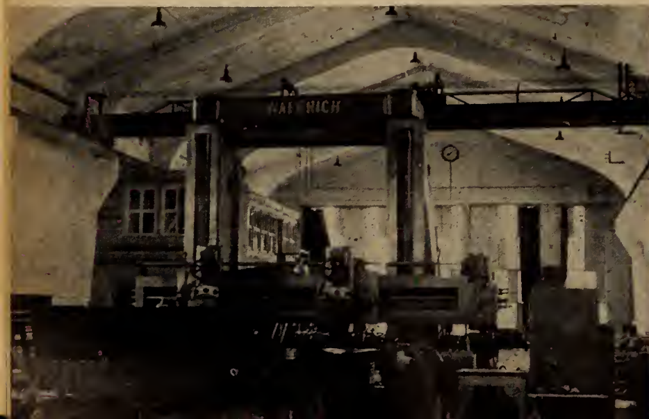
Fig. 11. Large planing machine in central workshops at L.F.A.
