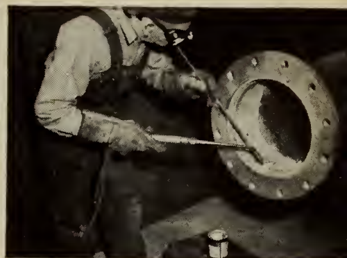
Flanges are quickly joined to cast iron pipe sections by bronze-welding. DOC supplies several bronze rods to meet varying service requirements.
