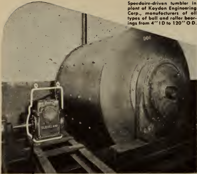
The white outline on the photograph indicates the much larger size of standard drive required to do the work of Speedaire.
