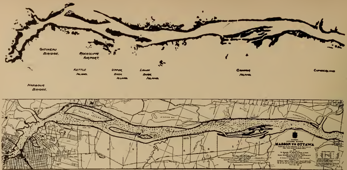
Fig. 9. Radar mosaic of Ottawa River, (composed from MMR display) with map of corresponding area.
