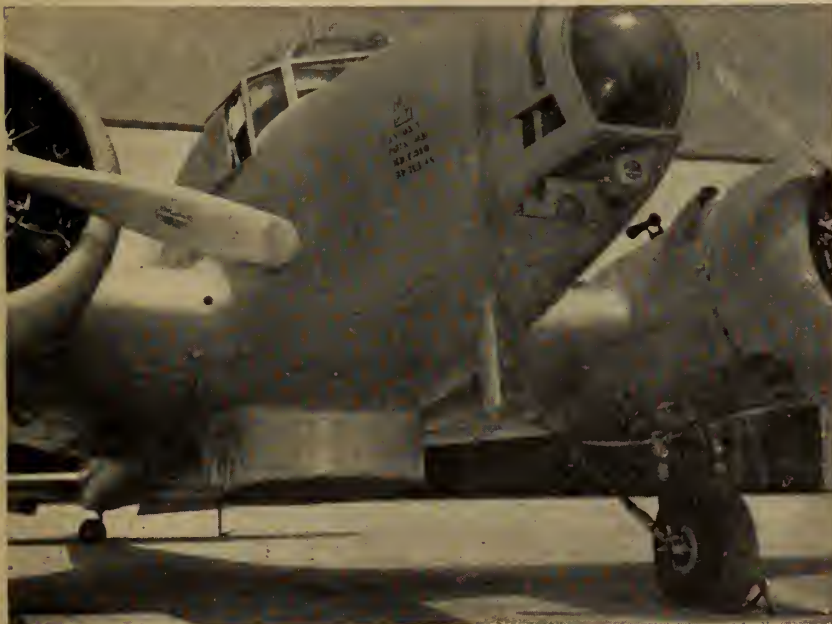
Fig. 12. Altimeter antenna mounted on aircraft.
