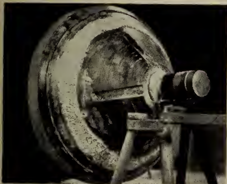
Bronze-welding this cast steel cone crusher head saved $1,000. The crack, which ran completely around the head for a distance of 9½ ft., extended through the thickness of the casting in several places. It was veed out by flame-gouging.
