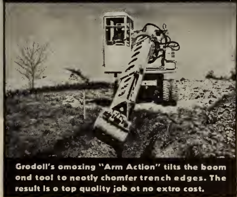
Fast, telescoping action of boom makes digging and loading one continuous operation... loading out dirt in record breaking time.
