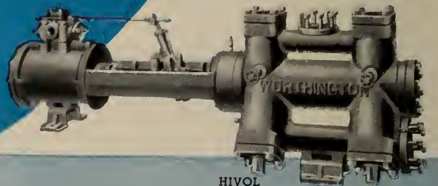
HIVOL Horizontal Simplex Direct-Acting Piston Pump for refinery service, for discharge pressure up to 400 p.s.i. An excellent pump for highly volatile liquids and high volumetric efficiencies.
