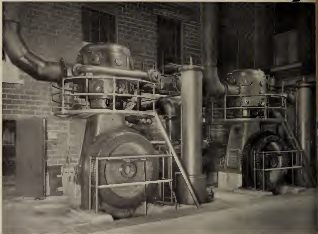
Night and day these two 14½" stroke XVHE-2 Air Compressors deliver over 5000 c.f.m. of Air Power at 100 lbs. pressure.
