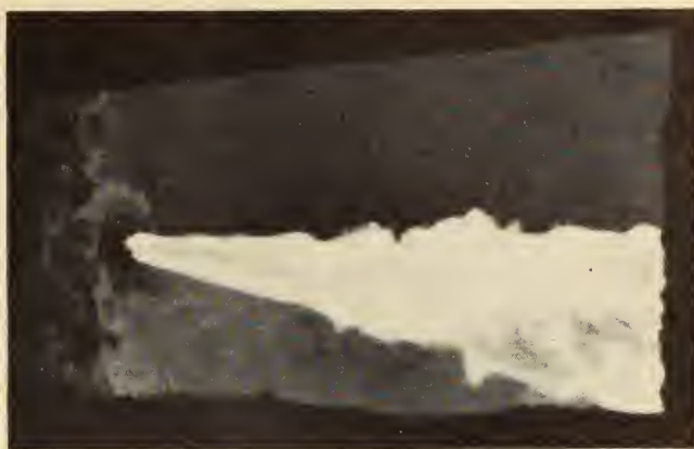
Fig. 1—Open hearth flame without oxygen.
