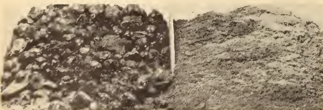
Fig. 4—Granulated open hearth tapping slag. At left—as granulated, coarse. At right—as ground to 80% minus mesh. For agricultural use.
