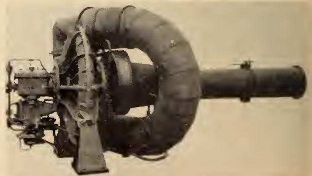
Fig. 1. Whittle's first experimental engine—1937. Photo reprinted from Proceedings of Institute of Mechanical Engineers, courtesy British Thomson Houston Company.
