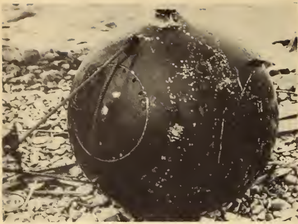
Fig. 9—Type "O" German magnetic mine.
