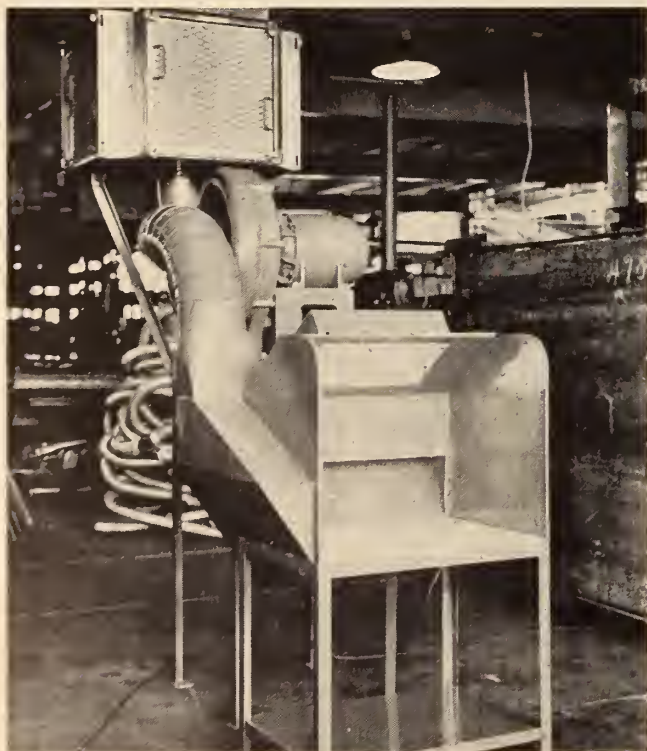
Fig. 2. Portable grinding stand with booth-type enclosure and air-recirculating dust collector. Courtesy American Air Filter Company, Louisville.
