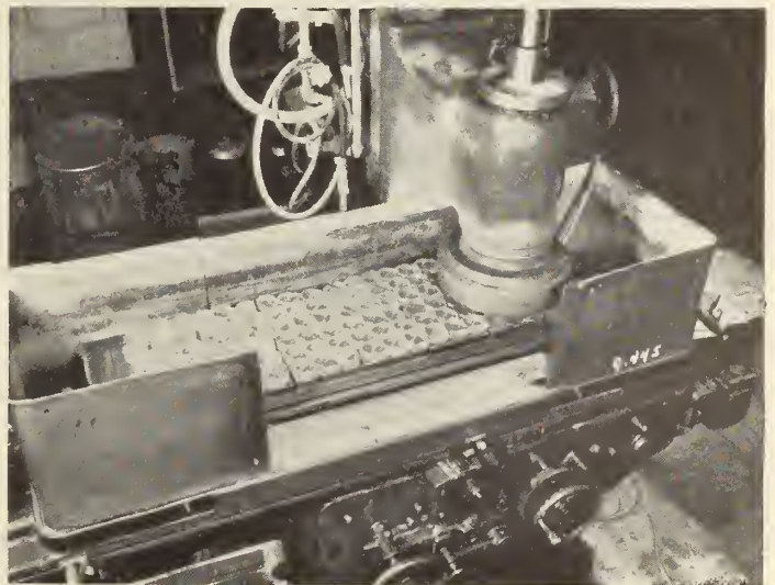
Fig. 14—Pratt & Whitney prism milling machine with 14" diameter diamond cutter.
