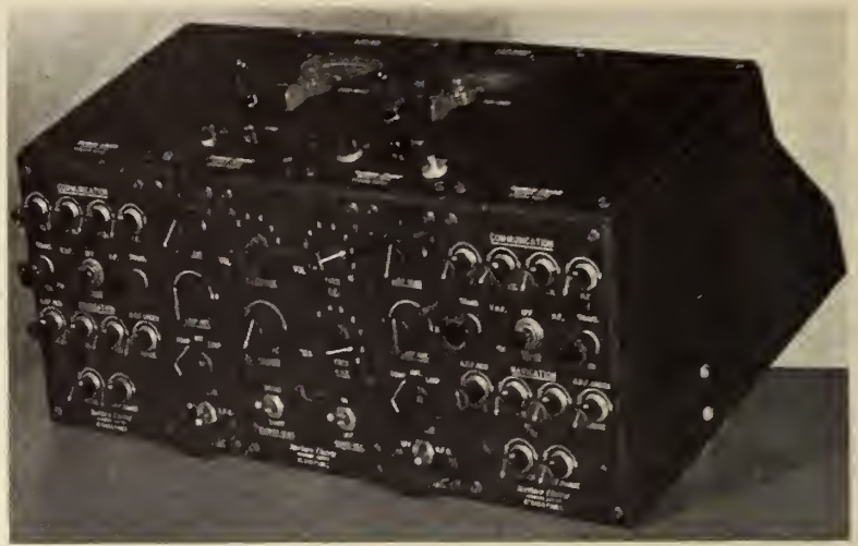
Fig. 6—Radio control pedestal designed for TCA for the DC-4M DeLuxe airliners being built by Canadair in Montreal.
