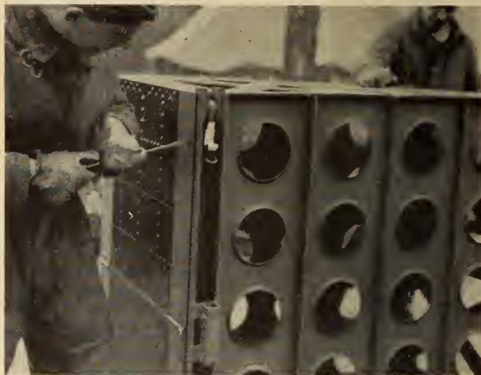
Fig. 7—Final stage in assembly of a standard bay. Dzus fasteners are locked in position throughout.
