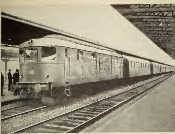
Fig. 5—Passenger train driven by first gas-turbine locomotive at Gare de l'Est in Paris.
