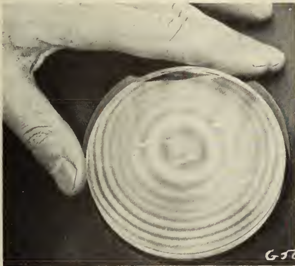
Fig. 9—Showing the appearance of interference rings between lens and test glass.
