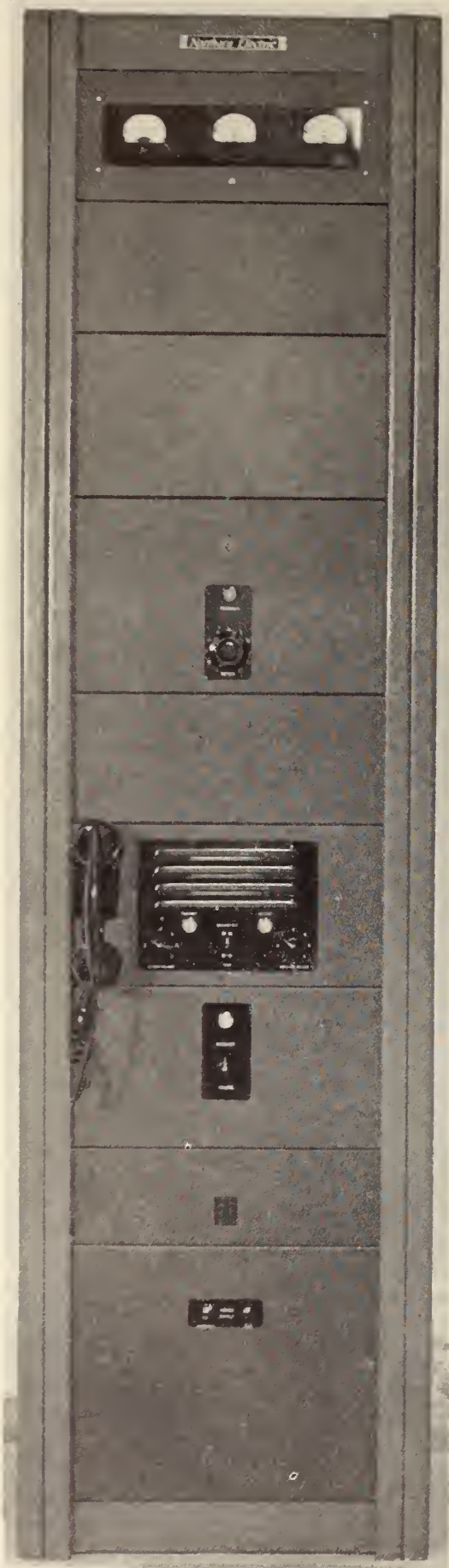
Fig. 10—Power line carrier terminal.
