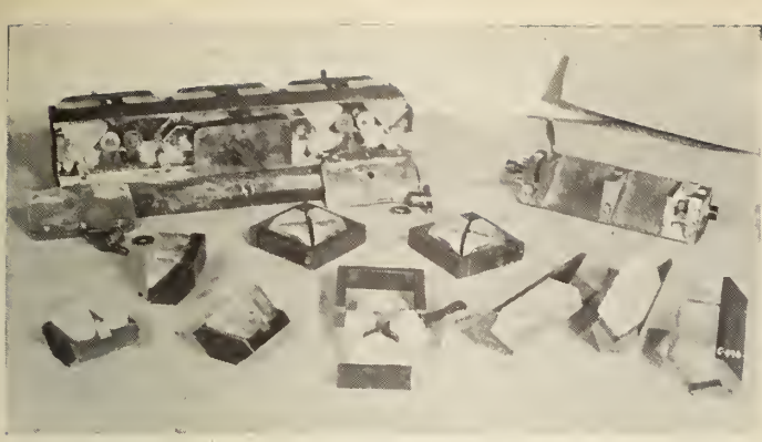
Fig. 16—A group of mechanical holding fixtures for prism milling.
