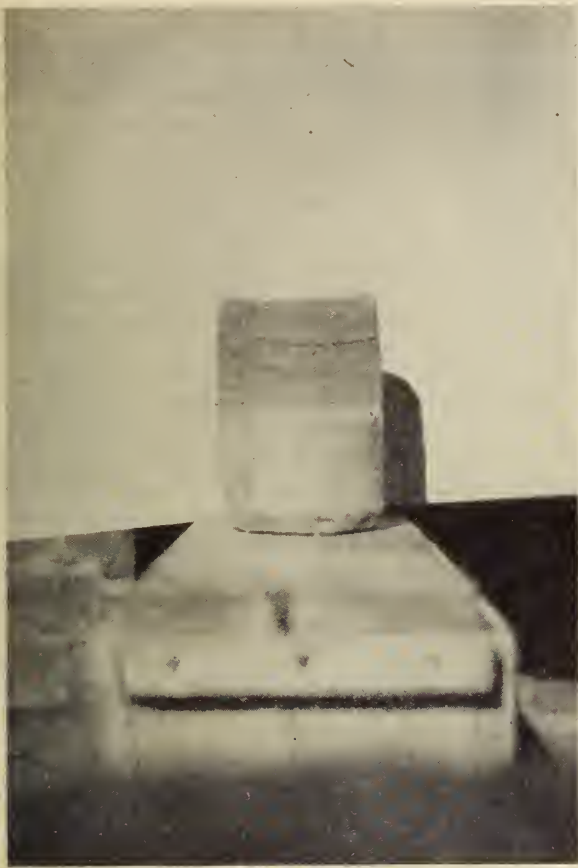
Fig. 2—Ice lens produced in the laboratory.
