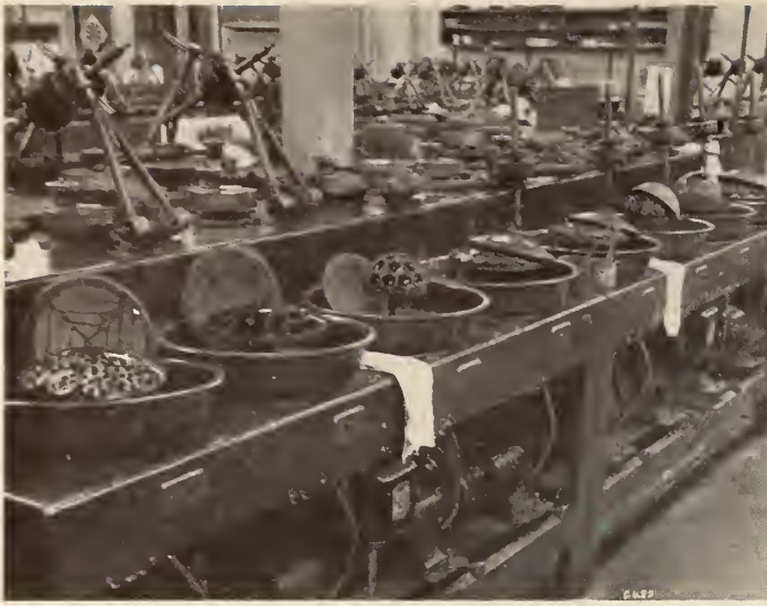
Fig. 11—A typical lens polishing machine for large blocks.
