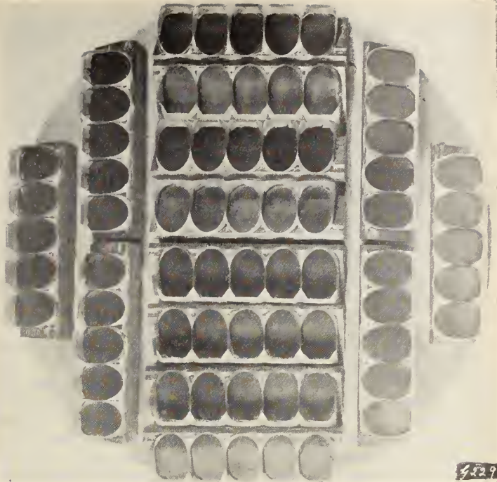
Fig. 19—Block of 70 binocular prisms on steel angle bodies.
