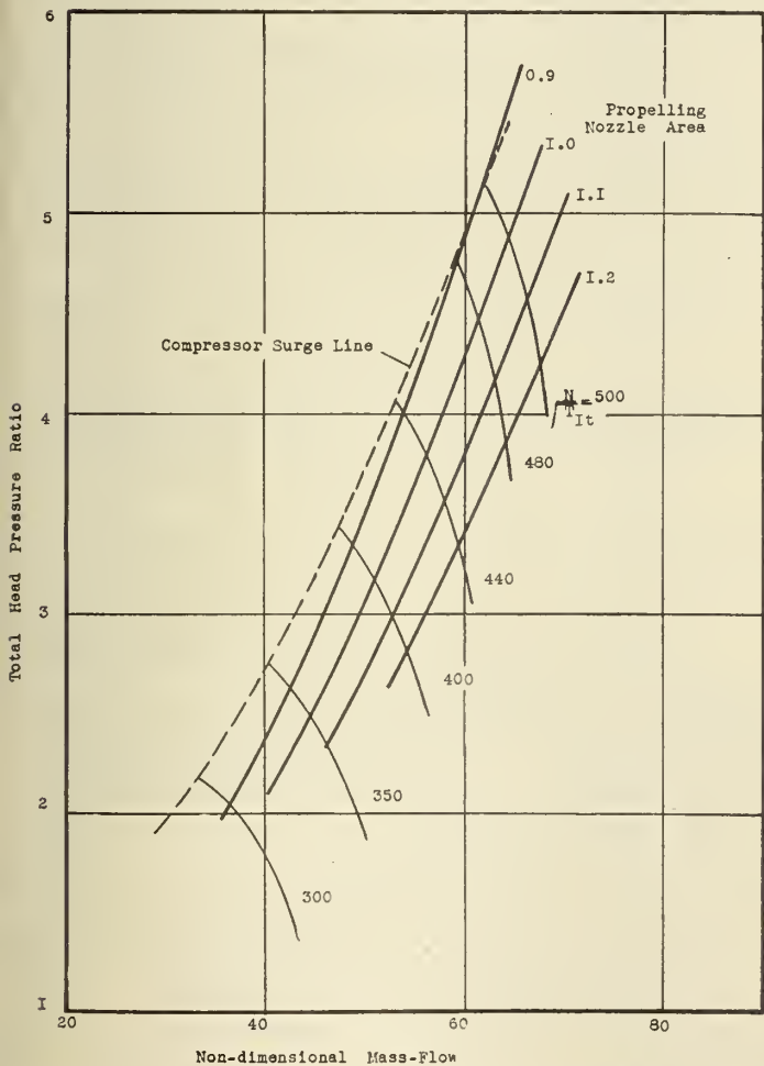
Fig. 32—Equilibrium running characteristics of a simple jet with variable propelling nozzle.
