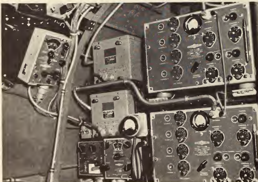
Fig. 5—Wireless operator's table, Lancaster bomber, showing TA-12 transmitters with associated antenna loading units, MR9 remote control for R-10 receiver, MN-28 remote control for MN-26 compass receiver, and 3616-B transmitter control.
