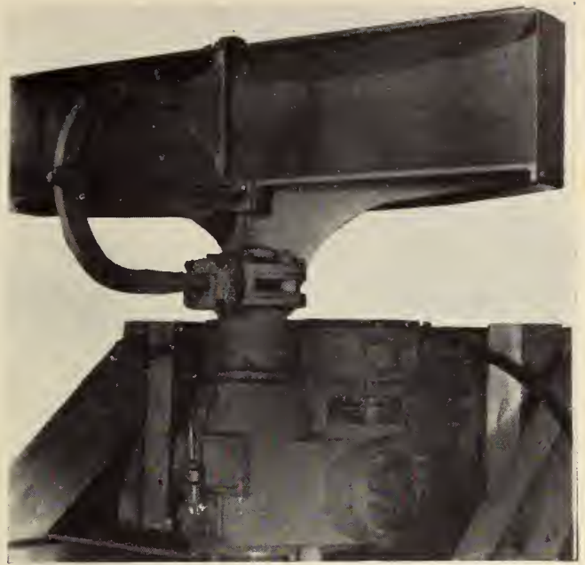
Fig. 8—Microwave search antenna used with 268 naval radar equipment.
