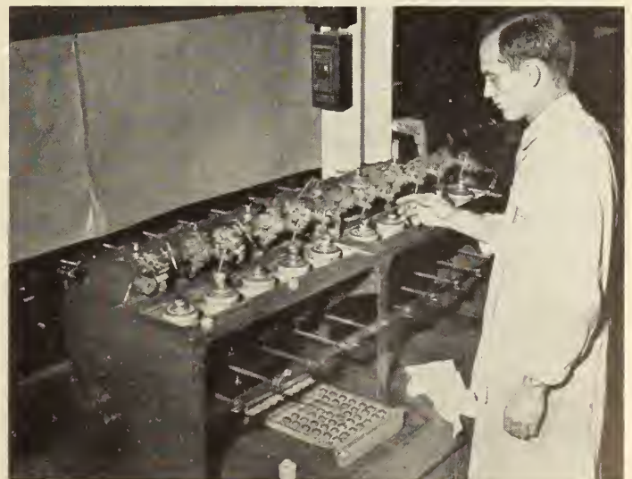
Fig. 10—A typical single lens polishing machine.
