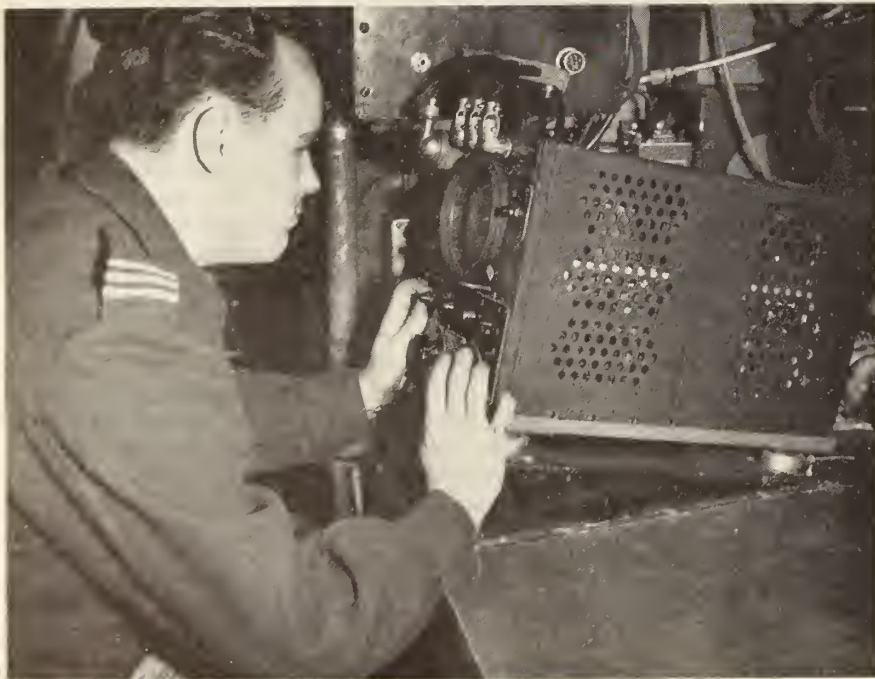
Loran equipment installed in T.C.A. planes operating on the trans-Atlantic route.
