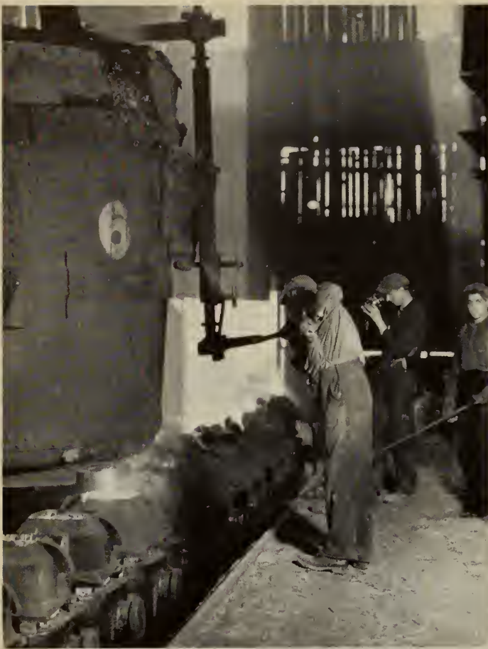
Fig. 5—Pouring Steel into Moulds.
