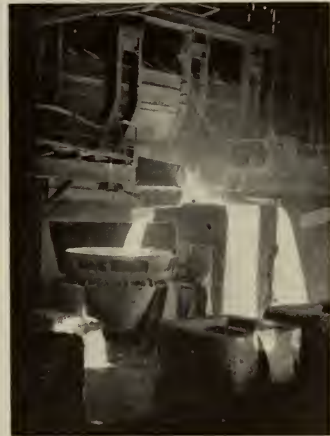
Fig. 4—End of Tapping showing Slag running out of Ladle.
