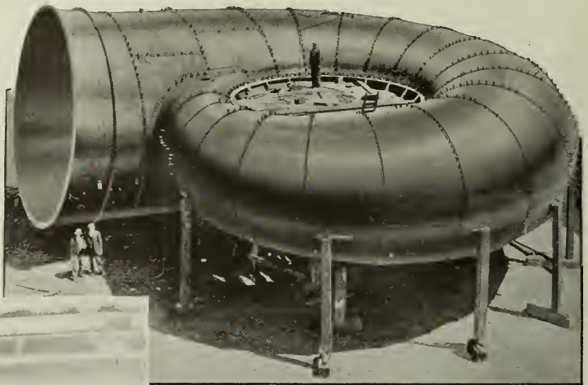
Volute Casing, Intake Diameter 23 3"
