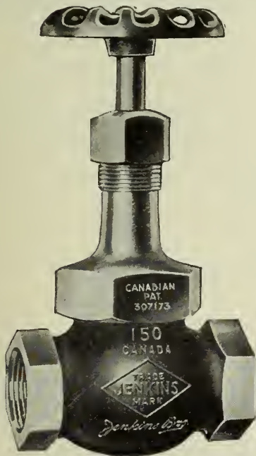
Fig. 106-A—Standard Bronze Globe Valve for 150 lbs. working steam pressure or 250 lbs. oil, water and gas working pressure. Has special exclusive Jenkins features, including one-piece screw-over bonnet and slip-on, stay-on disc holder.
