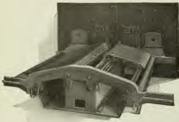
Rear view showing retort, grate bars, dump grates and auxiliary windbox.
