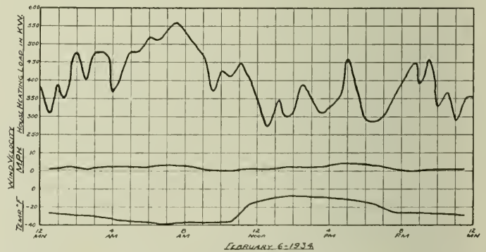
Fig. 4—Typical Residence Heating Load as Affected by Wind Velocity and Atmospheric Temperatures.
