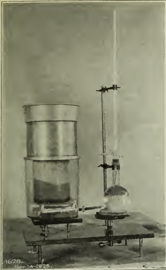
Figure No. 6.—Capillary Pore Determinator as Used on the Absorption Experiments of the Hydro-Electric Power Commission of Ontario.
