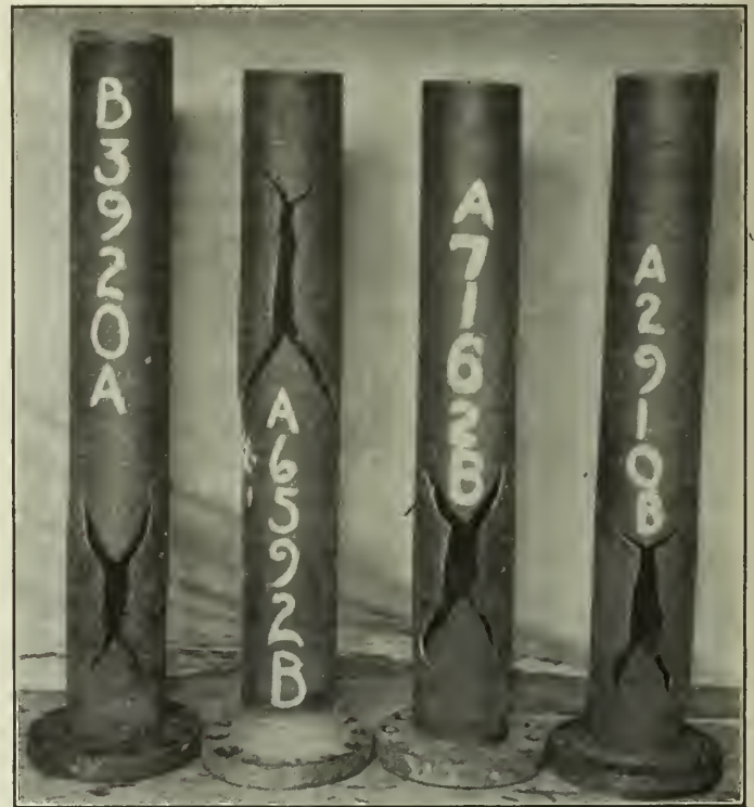
Figure No. 23.—Hydrostatic Pressure Tests on Selected Line of Pipe.
