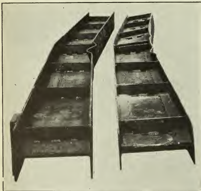
Figure No. 4.—Result of Test of Welded Plate Girder (with Plates and Angles).
