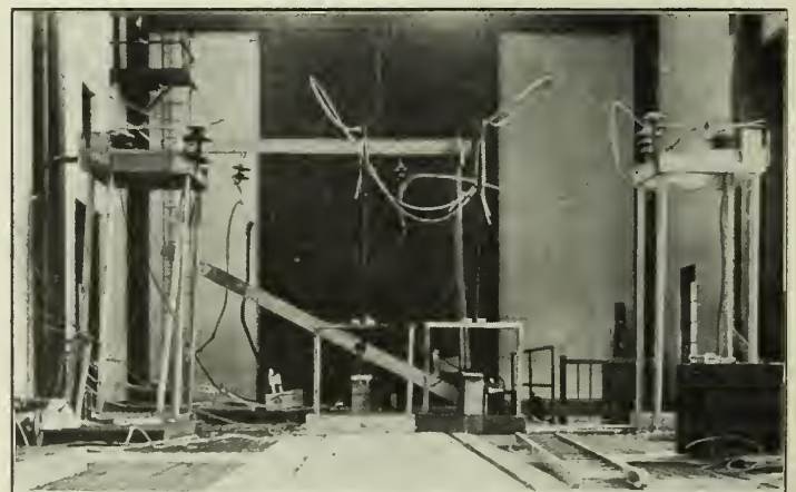
Figure No. 15.—View showing Structure and Loops over which Arcs were Formed.
