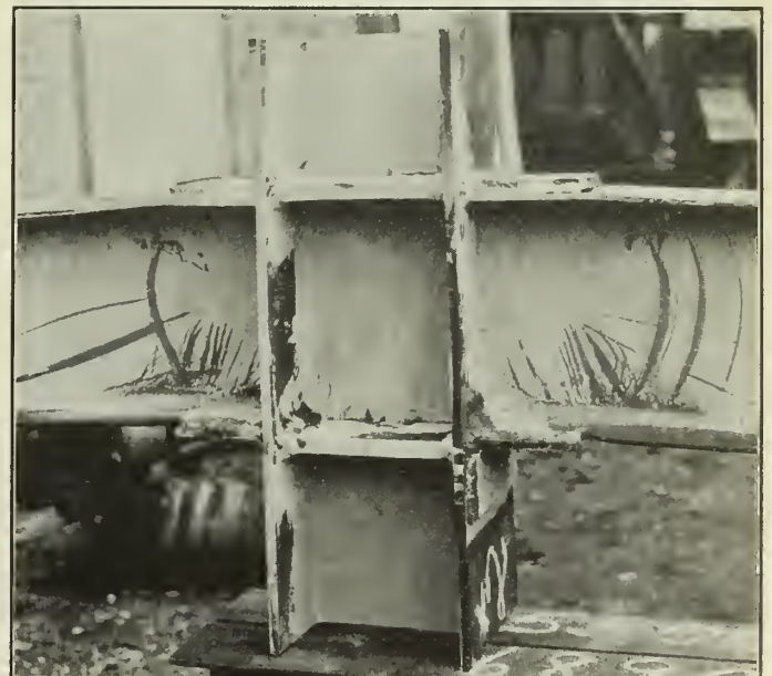
Figures Nos. 1 and 2.—Welded Cantilever Joint Used in Test at Carnegie Institute of Technology in Pittsburgh.
