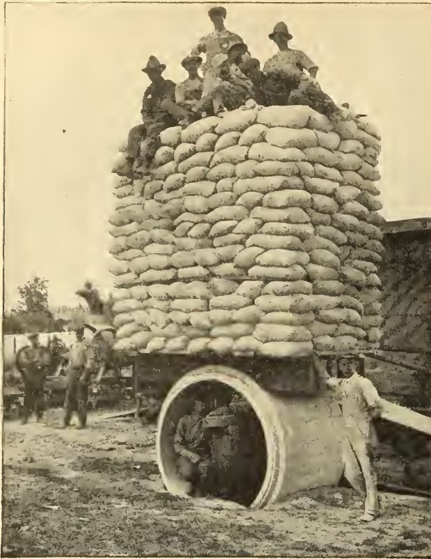
Testing 60-in. Concrete Pipe under a total weight of 42,000 lbs. Engineers estimate that this pipe would stand twice this pressure.
