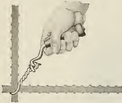
Illustrating ease with which Bates Bars Ties are applied
