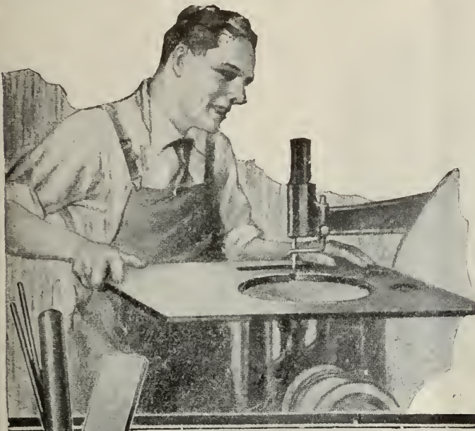
Cutting Fibre on a Band saw in the plant of the Diamond State Fibre Company.
