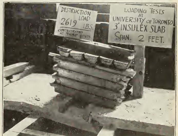
Figure No. 4.—Experiments at University of Toronto with Insulex, Puffed Gypsum.
