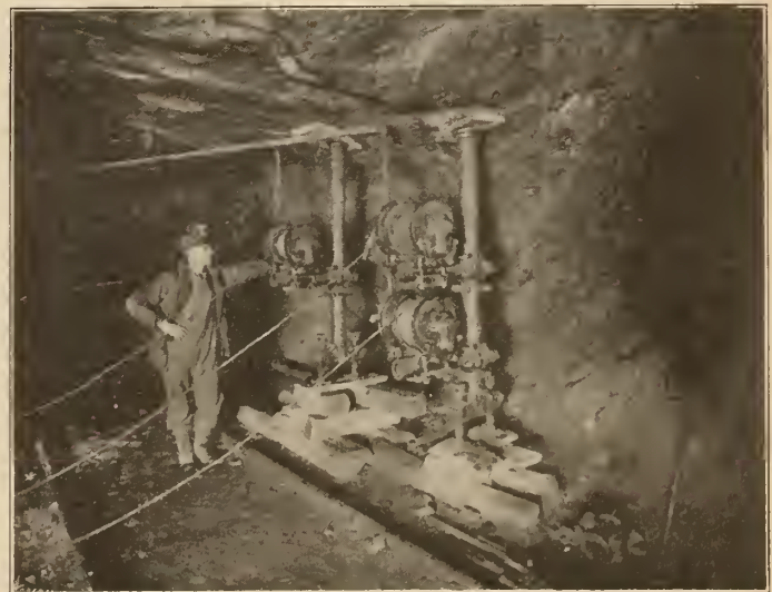
Plate No. 2.—Three little Tugger Hoists installed for hauling a 12,000-pound loaded Car of Rock up a Rock Tunnel driven in the Mine of a large Coal Company.
