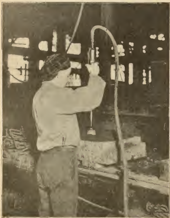
Plate No. 4.—Ramming Sand for small Mold with a Bench Type Pneumatic Sand Rammer in a Canadian Foundry.
