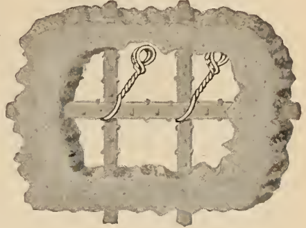
Sectional View showing Reinforced Bars held in place by Bates Wire Ties.
