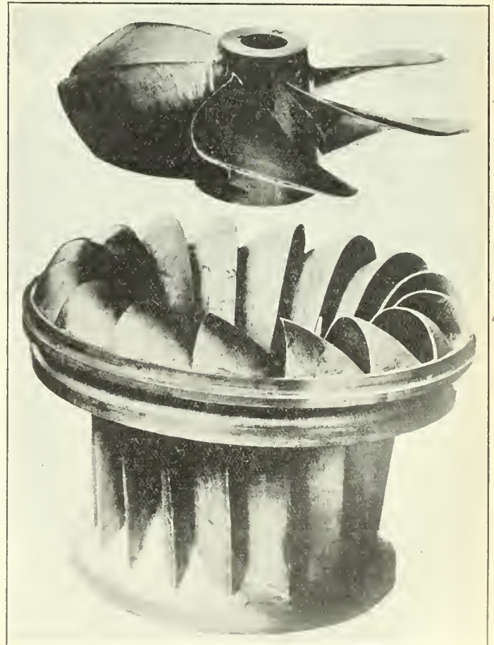
Figure No. 3. Comparison between Propeller and Francis Types of Turbine Runners.
