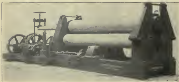
Fig. 10.—Motor Driven Plate Rolls.
