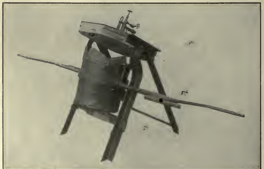
Fig. 3.—New Form of Ladle Heater Recently Placed on the Market by the Monarch Engineering and Manufacturing Co.
