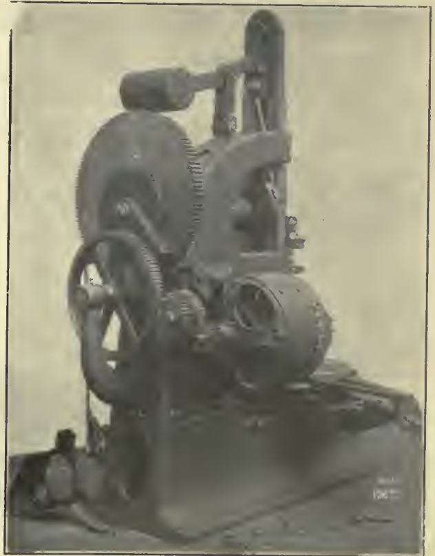
Fig. 13.—12" Slotter With Link Slotting Attachment.
