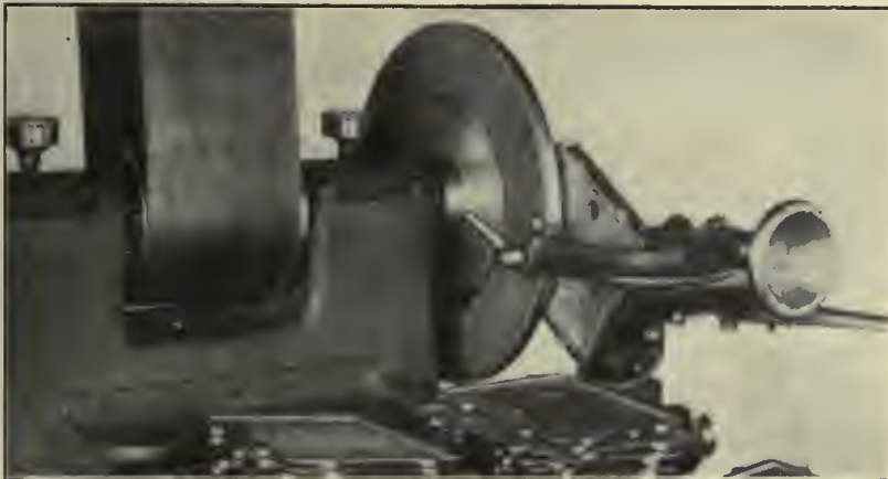
Fig. 1.—Grinding Jacket Plates, Showing Special Jig.
