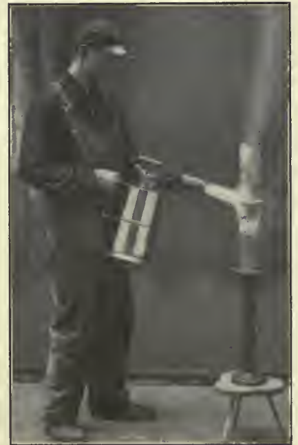
Brazing a Cup Joint With Kerosene Lamp.
