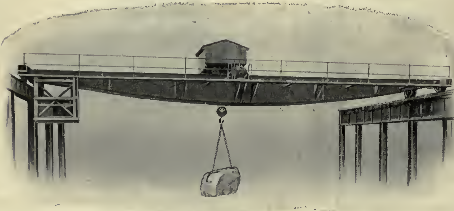
Photo of 5-toni Motor Travelling Crane, 60-foot span
