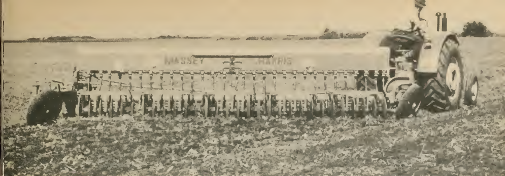
The one-way disc harrow and seeder is a relatively new implement. Though trash cover is light on this field the "discer" is adapted for conserving cover.
