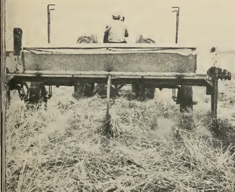
New-type drill designed and built by an ingenious farmer for the purpose of placing seed in the ground beneath heavy trash cover. This machine is still in experimental stage. At right, bar of drill is bared to show how it operates.
