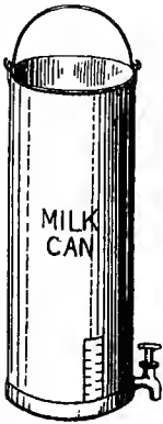
CAN FOR DEEP-SETTING OF MILK.
