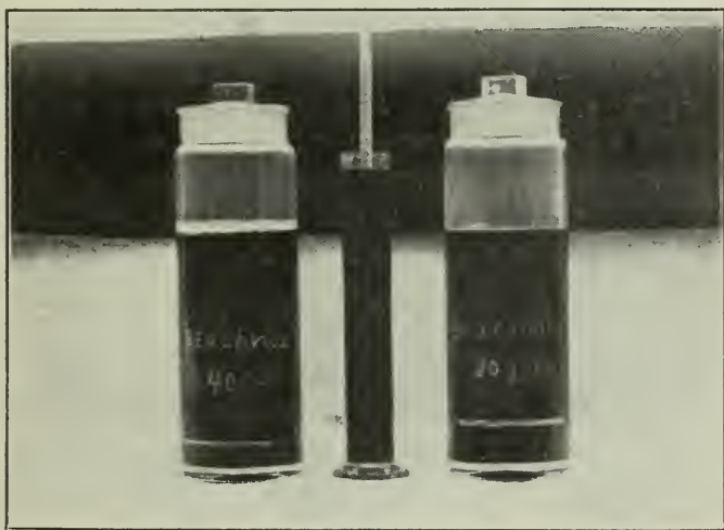
Fig. 7. (a) Shows the comparative amounts of sediment from boiling the same proportions of lime and sulphur in 40 and 30 gals. respectively. Note the larger amount of sediment in the latter case, thus showing the importance of keeping the water up to at least the 40 gal. mark. (b) Hydrometer in glass cylinder of the liquid.
