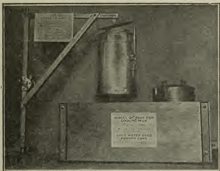
TANK FOR COOLING MILK AND HOISTING APPARATUS.
