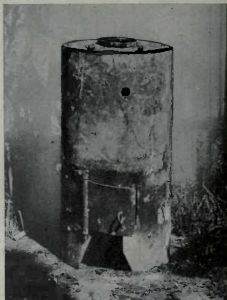
SALAMANDER, OR PLASTERERS' STOVE; STOVES SOMEWHAT SMALLER WERE USED IN EXPERIMENT. (ORIGINAL).
