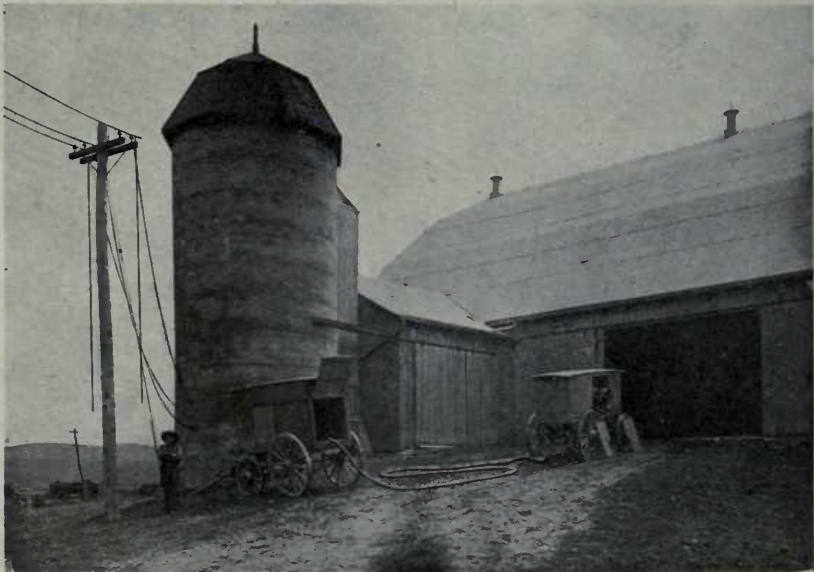
VIEW OF SYNDICATE OUTFIT SHOWING MOTOR AND TRANSFORMER WAGONS. ONE TRANSFORMER IS CONNECTED TO THE LINE AND SUPPLIES CURRENT TO THE MOTOR AT SUITABLE VOLTAGE
