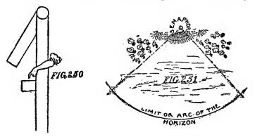
nalling exactly as the arms of a man when doing the same service, the semaphore of course, is set at a point where it may be seen the greatest and also the widest distance, or to put it more scientifically the semaphore is set at a point "so situated that it may be seen through the greatest arc of the horizon" (Fig. 251).
