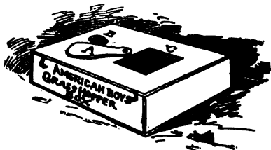
FIG. 90.—A, the sliding door; B, the grasshopper hole; C, the air window protected by wire netting.
