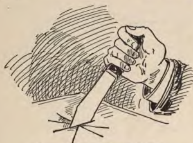
FIG. 19.—How the Tin is Cut.
