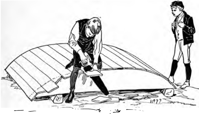
FIG. 29.—The Ends may be Sawed off Flush.
