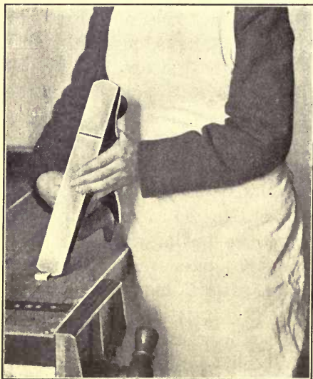
FIG. 25. — SETTING A PLANE.
