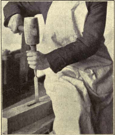
FIG. 122. — METHOD OF GRASPING THE CHISEL FOR MORTISING LARGE WORK.
