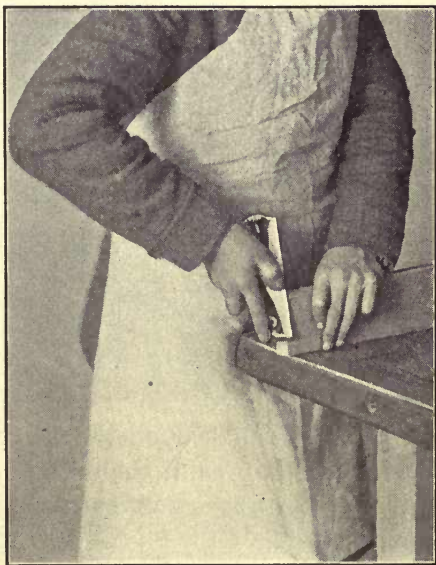
FIG. 34.—USING BLOCK PLANE UPON SMALL PIECES.
