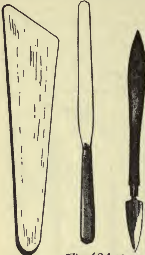
Fig. 180 Horn Palette- knife. Fig. 181 Fig. 182 Steel Palette- knife. Steel Scraper. (Reduced sizes.)
