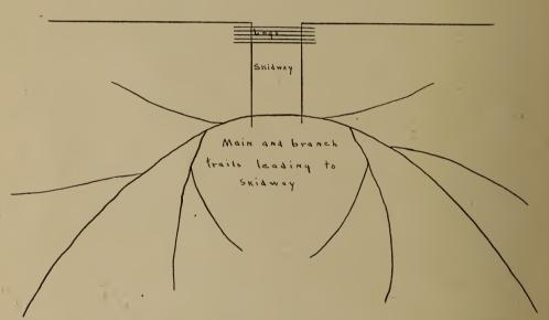
Drawing showing relation of skidway to main road, and of trails to skidway.
