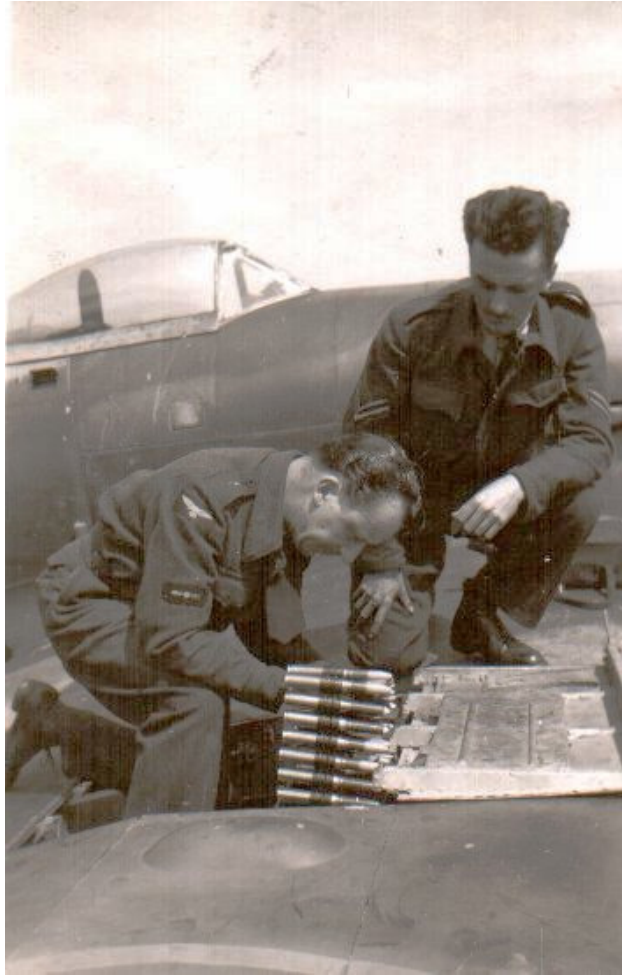
Figure 5.4: 'Corporal for a day'. HN's war album. 20mm ammunition being loaded. Is this Les Wilburn with the stripes? Note the size of the shells and the fact that the heads have different patterns. That is, some will be high explosive, some armour piercing, some tracer, etc.
