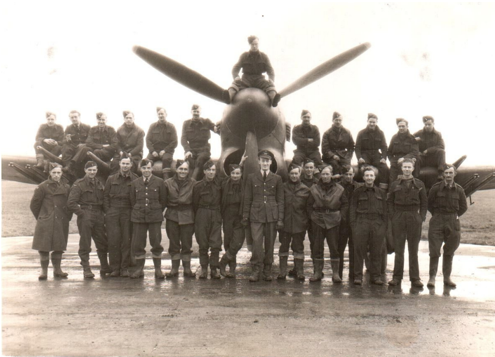
Figure 5.6: Section of 247 Squadron at Warmwell, Dorset, 1945. This is a 3-bladed propeller version of the Typhoon, which was gradually replaced in 1945 with 4-bladed versions. The rocket rails are clearly visible. Harry is third from right, front row.
