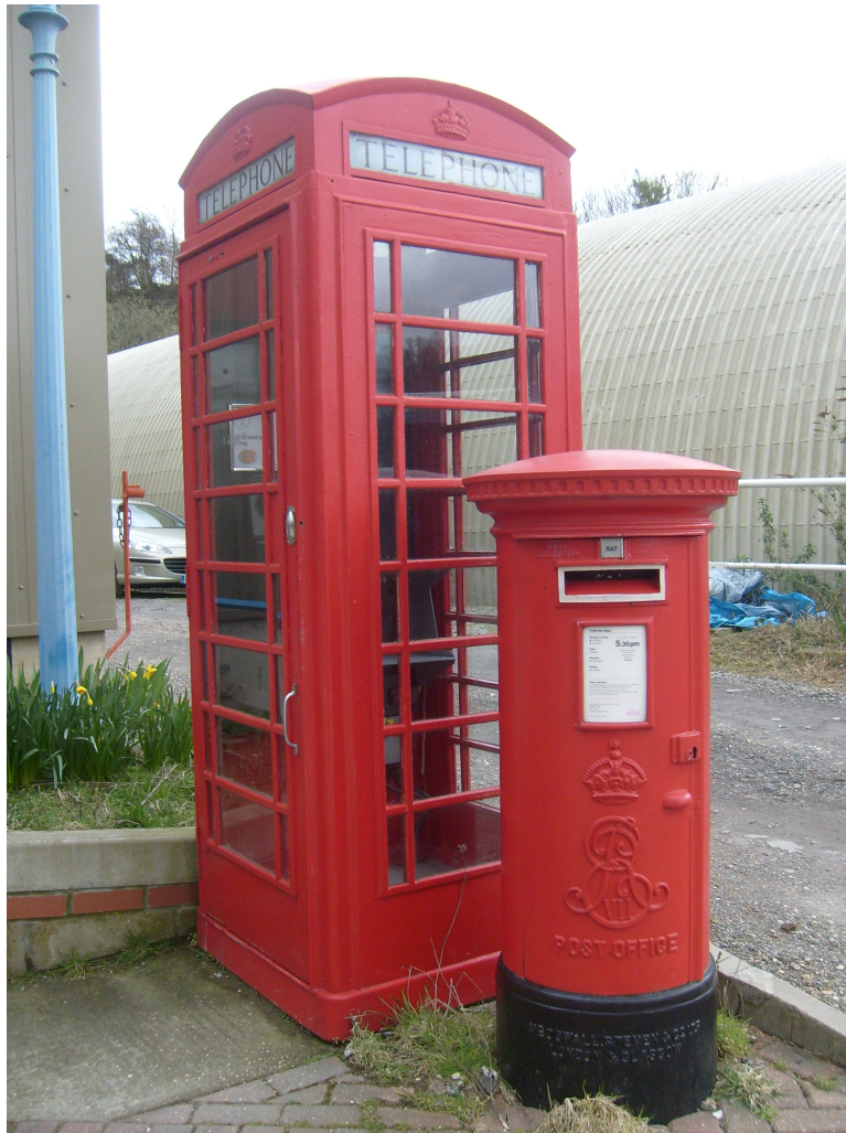
Figure 14.7: A K6 telephone box and Edward VII pillar box at the Amberley Working Museum. Source: Wikimedia Commons. To operate, one put in money, dialed or requested number, and when the called party answered, one would push button A to connect, or button B to send money to the refund chute. Both buttons had about a 1.5 cm. action and were quite heavy to depress. I believe it was 2d. for a local call (2 old pence).
