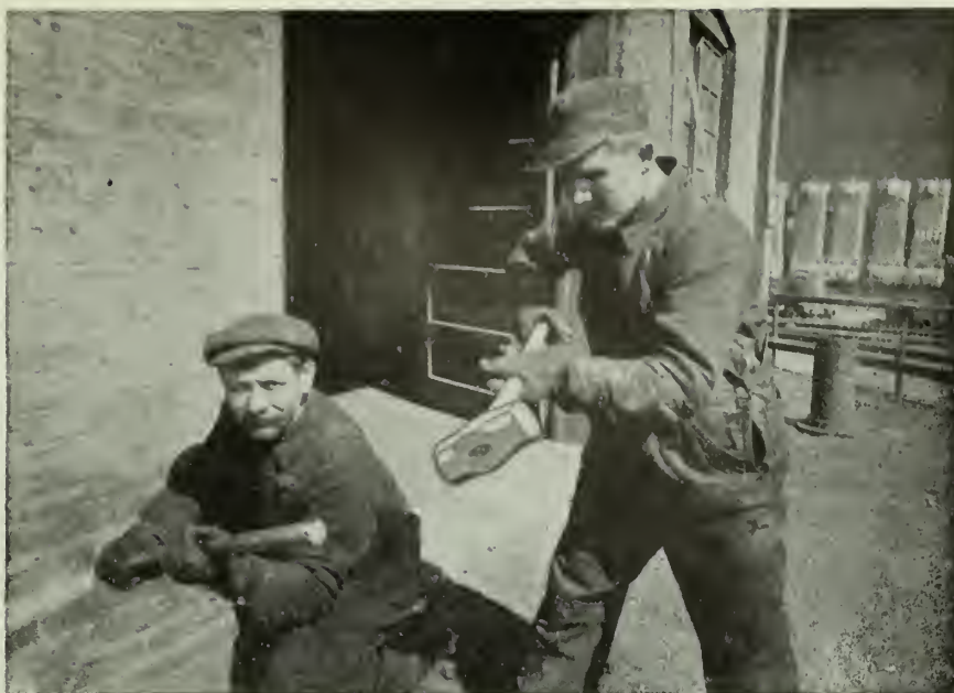
FIG. 31. UNSAFE WAY OF HOLDING BAR FOR A SLEDGE. MAN HOLDING BAR IS ON SAME SIDE AS STRIKER.
