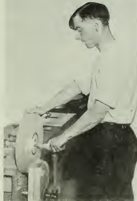
FIG. 2. REBUSHING GRINDING WHEELS.
