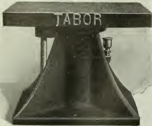
3" Tabor Jarring Machine with 12" x 14" Table.
