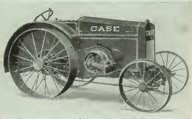
CASE 9-18 AUTOMOBILE TYPE TRACTOR WITH 4-CYLINDER MOTOR PLACED TRANSVERSELY.
