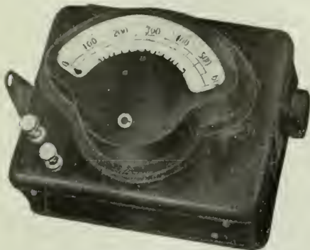
CASE CONTAINING BATTERY, RHEOSTAT AND MILLI-AMMETER FOR USE WITH OPTICAL PYROMETER.
