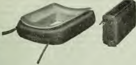
FIG. 4 SHUNT FIELD COIL ON ALUMINUM, ALSO INTERPOLE COIL.
