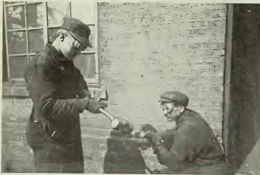
FIG. 32. SAFEST METHOD OF HOLDING A BAR.
