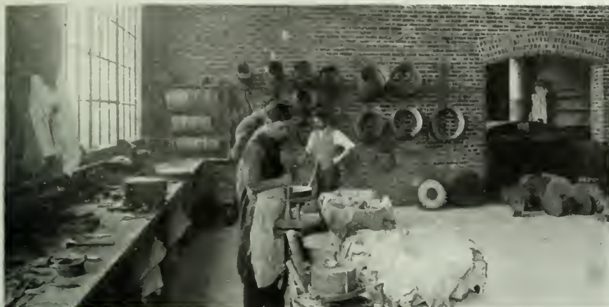
SILICATE PROCESS DEPARTMENT SHOWING TAMPING STOOLS, WHEEL MOULDS AND OVEN IN BACKGROUND.
