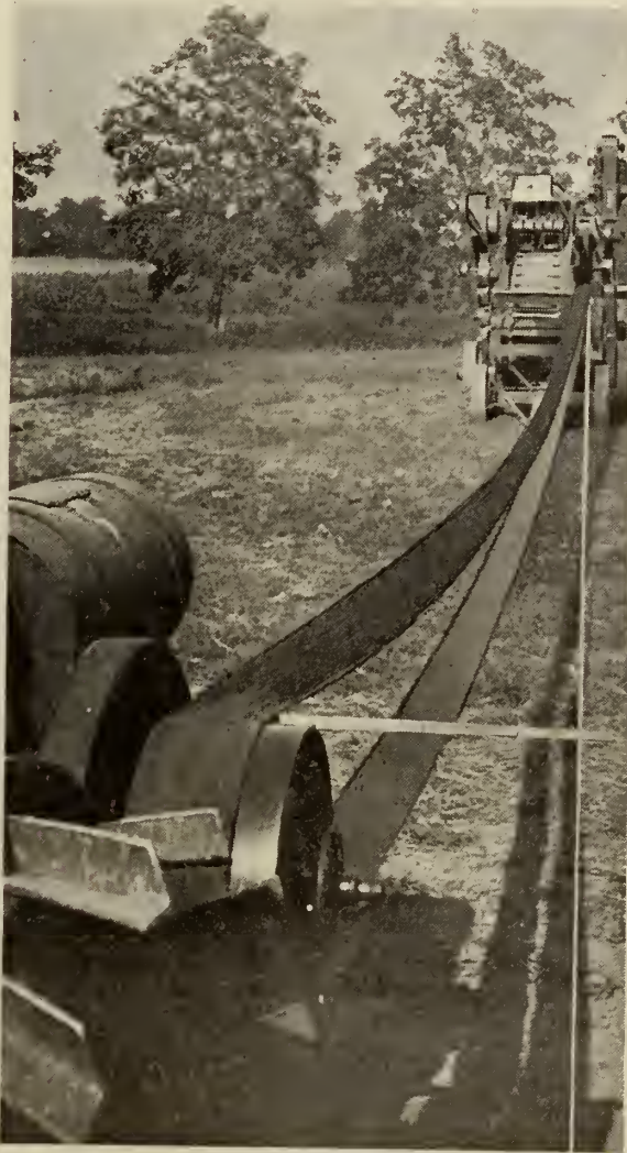
Tractor placed nearly 18 inches out of line, but front end turned to right as in No. 4 of diagram—to show that because belt runs to left, the tractor is not necessarily too far to right.
