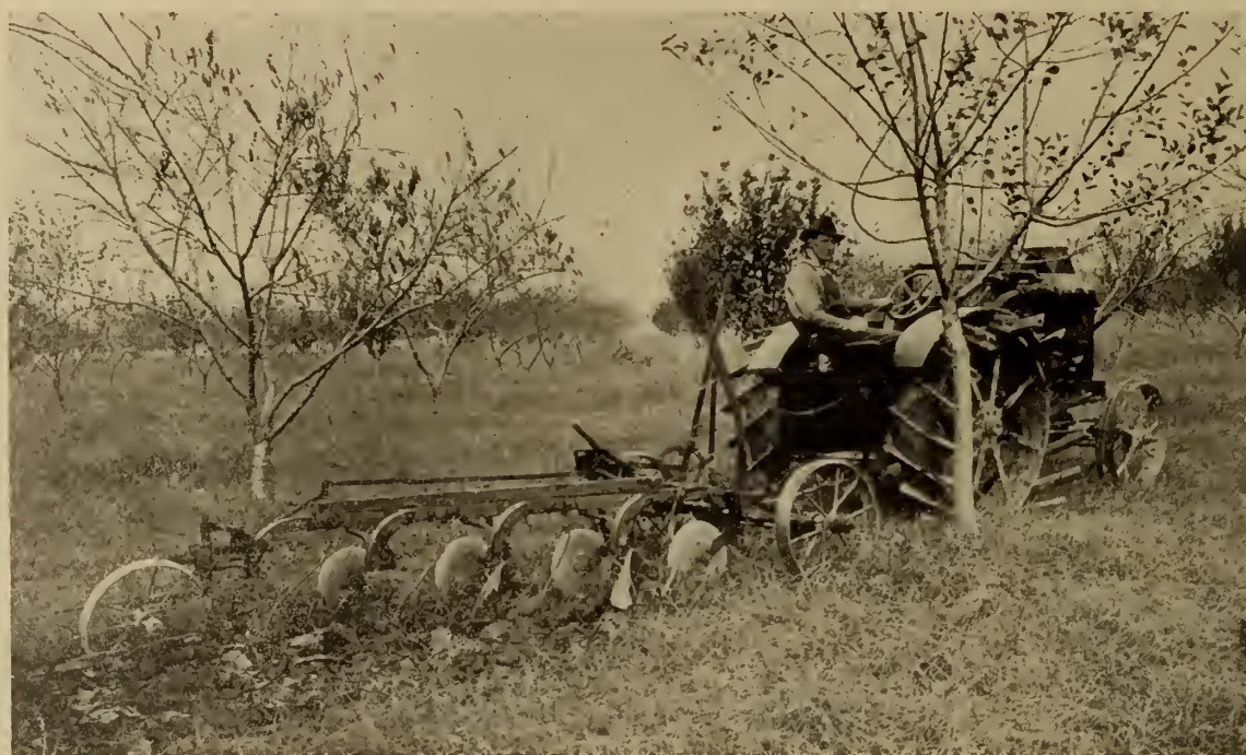
A New Jersey farmer pulling four 14-in. bottoms with a 12-20 Advance Rumely tractor in very light soil.
