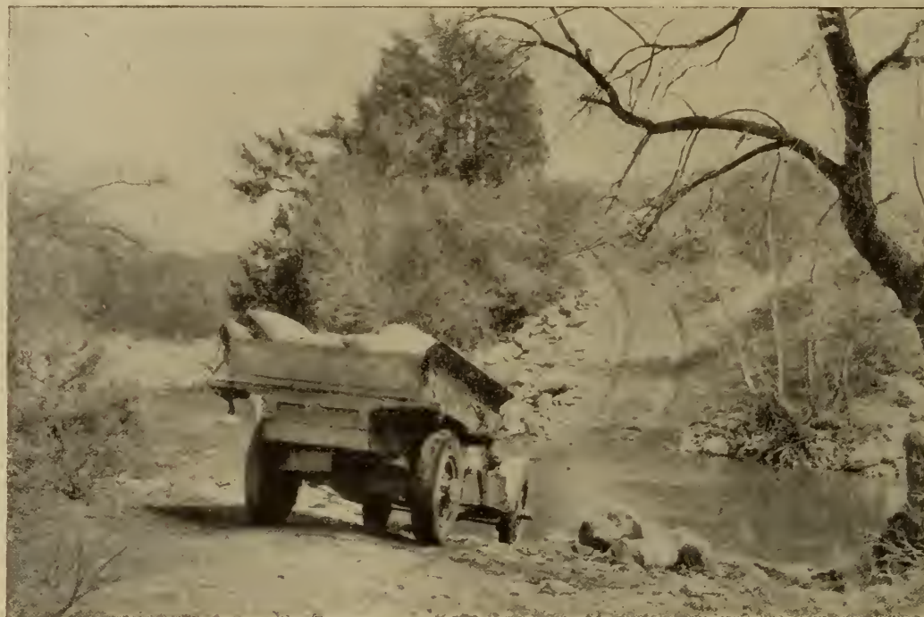
A farm truck, equipped with pneumatic tires, starting to ford a creek and haul its load over the worst kind of roads. Truck engineers estimate the saving of fuel consumption with pneumatics at from 15 to 30%.
