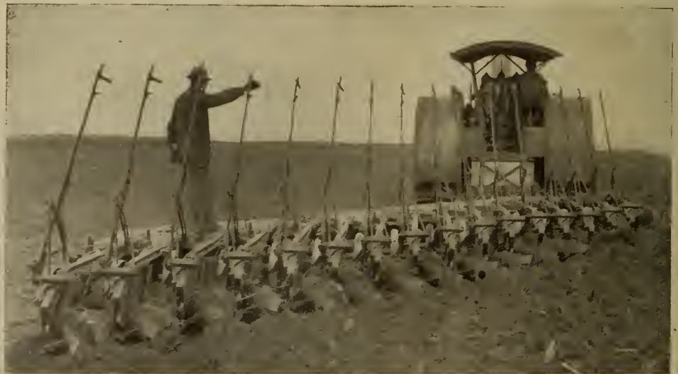
30-60 Fairbanks-Morse Oil Tractor pulling sixteen 14-inch plows in corn stubble at a test. This plow turns over a strip of land 20 feet wide every time it goes down the field.
