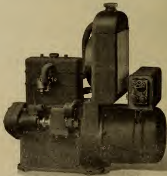
Kohler Farm Lighting Plant.
