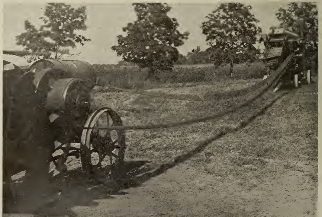
This shows effects of running belt twisted over pulleys out of line. One edge badly stretched so that the belt does not hang flat.
