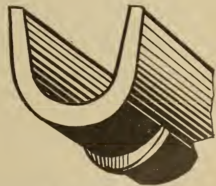
Section of Post, showing actual size: Note unusual thickness.
