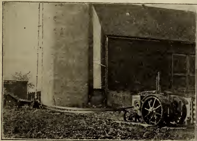
A tractor sale also means the sale of a belt-power machine to go with the tractor. Illustration shows a tractor operating ensilage cutter and silo filler.
