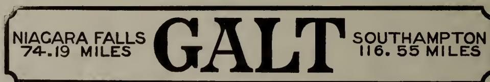
Style no. 2, as used on the Grand Trunk Ry. System. Black letters on white ground. This sign is 14 ins. high by 7 ft. long. Length varies with number of letters in name of station.
