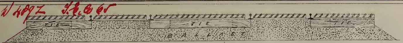
SECTION OF G.T.R. STANDARD SURFACE SLAT CATTLE GUARD.
