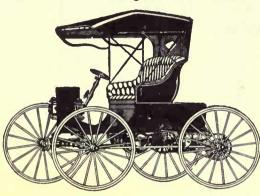
It is cheaper to feed gasoline to a Tudhope-McIntyre, than to feed oats to a horse. This \$550. Motor Carriage runs 30 miles on one gallon of gasoline and travels from 3 to 25 miles an hour. 12-14 horse power, double cylinder motor and solid rubber tires will carry you up any hill—over any road—in any kind of weather. Simple and Safe to operate. Complete with Chapman double ball bearing axles, solid rubber tires, horn, and three lamps—\$550. (Top with roll front, \$30 extra.
