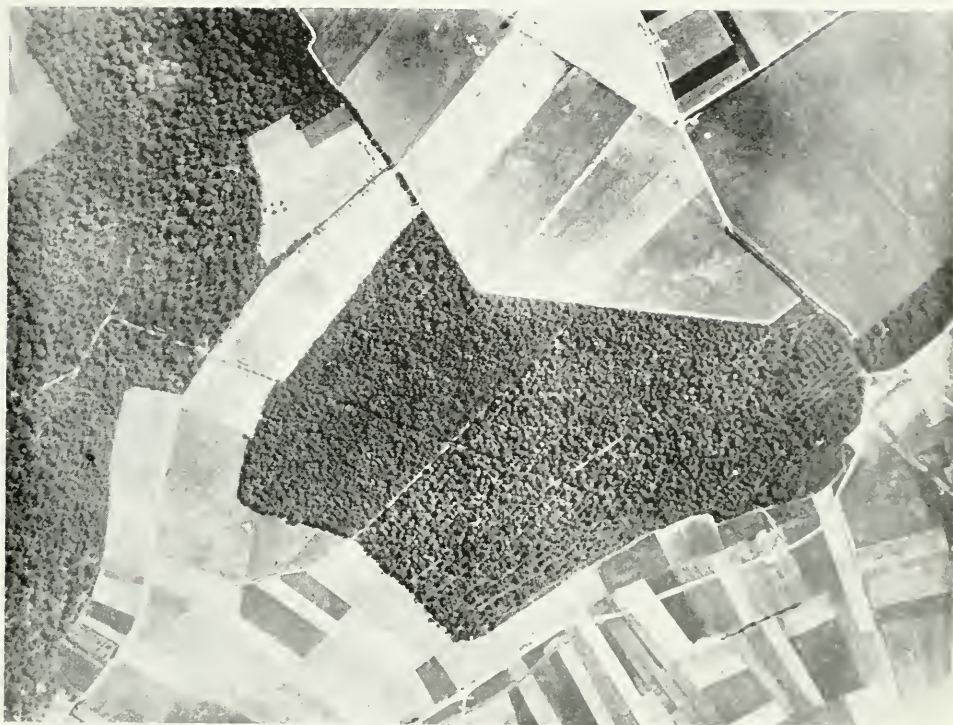
How wooded areas are defined by camera from 15,000 feet in the air. The strips of white and grey in blocks represent cultivated land, the difference in shading being accounted for by various crops, hay, grain, stooked and uncut fields, meadow, etc.
