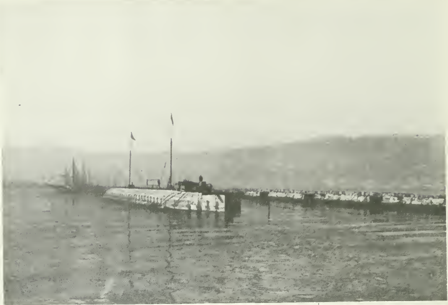
A new timber raft, built by a Canadian at Hommelvik, Norway, 360 feet long, 42 feet beam, 18 feet deep, which outrode a heavy gale in the North Sea. The possibilities of dispensing with ship bottoms in the transport of timber is engaging the attention of Canadian timber exporters.
