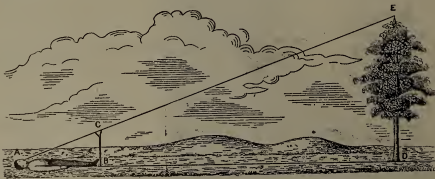
FIG. 2.—MEASURING HEIGHT OF TREE BY USE OF KNOWN HEIGHT TO EYE OF OBSERVER.
