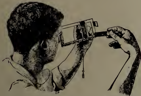
FIG. 4.—MANNER OF USING FAUSTMANN'S HEIGHT MEASURE.
