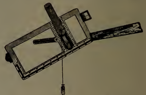
FIG. 3.—FAUSTMANN'S HEIGHT MEASURE.
