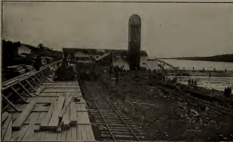
LUMBERING IN NEWFOUNDLAND—VIEW OF MILLERTON MILLS, SHOWING LIVE ROLLS CONVEYING LUMBER TO YARD.
