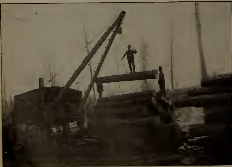
MONTANA : THE "MCGIFFERT" MACHINE THAT LOADED 215,000 FEET OF LOGS IN EIGHT HOURS. Observe the few men required in its operation.
