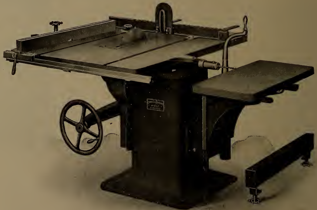
IMPROVED VARIETY SAW MANUFACTURED BY COWAN & COMPANY, GALT, ONT.
