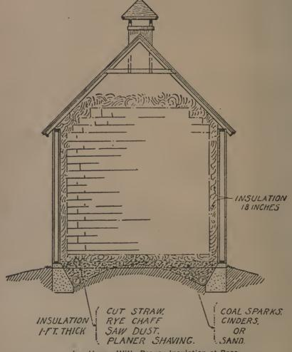
Ice House With Proper Insulation at Base.
