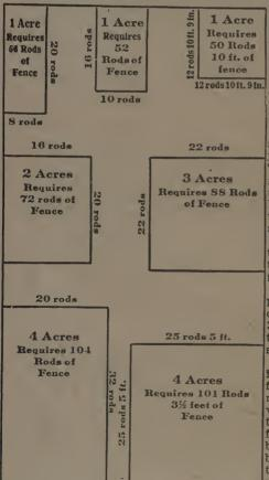
Dimensions given are exact, so that in buying ticle of earth in filling the holes, so fence, sufficient allowance should be made to that the posts will be as solid as a cover fence taken up in wrapping around end and tree. The second or brace post, also corner posts.
