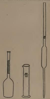
From left to right: Graduated Bottle Acid Measure and Pipette, used in Babcock Test.
