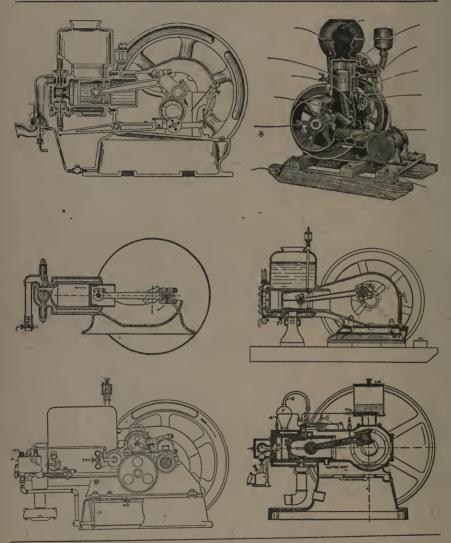
Five of these engines are of the horizontal and the sixth vertical. One thing in common that will be noticed is that all the cylinders are single acting. In one engine the rim of the fly wheel is simply indicated by a line. No attempt will be made to make comparisons, nor will space allow a lengthy discussion. Elsewhere
