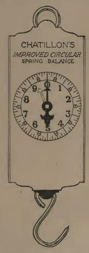
These scales will weigh 30-60 ibs. and have a loose pointer which by means of a thumb screw on the centre may be set anywhere on the dial, thus taking the tare of the milk pail. The price of these is given in test of dairy equipment.
