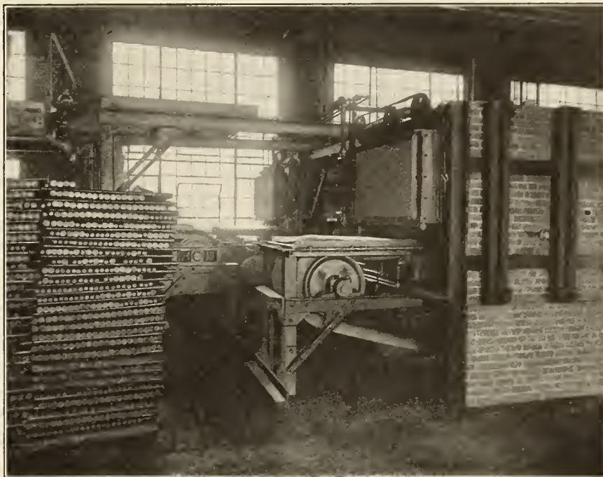
Automatic Tempering Furnace - Charging End For Rods, Bars, Shafts, Springs, Axles, etc.
