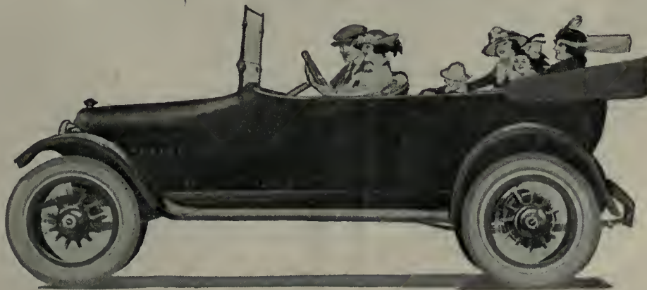
Model D-6-63 a new McLaughlin Six Cylinder Touring Car, 112 in. wheelbase 41 H.P. Valve-in-head Motor. A continuation of and improvement on Model D-60.
