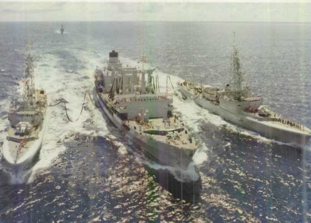
West coast ships refuel at sea from the tanks of HMCS Provider.
