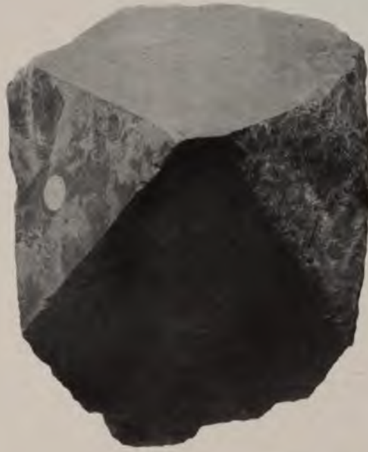
Crystals of Magnetite from Nepheline Syenite, Lot 30, Con. XV.—Faraday township. (Larger crystal weighs 7\frac{1}{4} lbs.)
