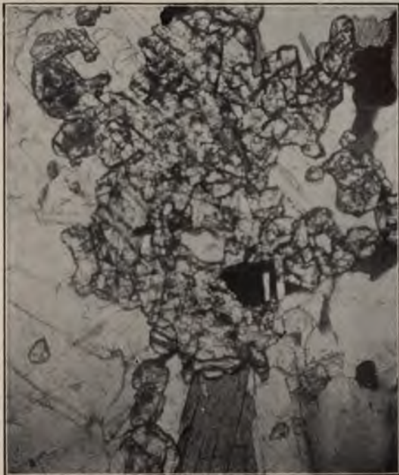
Corundum with Muscovite, Biotite and Plagioclase. Lot 2, Con. II.—Monteagle township. (x40 diam.)
