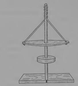
Fig. 137. Iroquois Pump-drill Fire-making Apparatus
