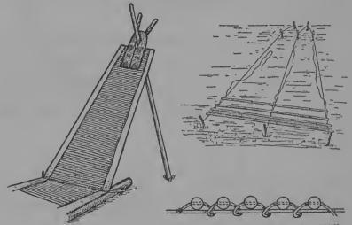
Fig. 79. Willow Bed or Back Rest Fig. 80. Frame for Weaving Willow Bed (AMNH) Fig. 81. Method of Fastening Rods
