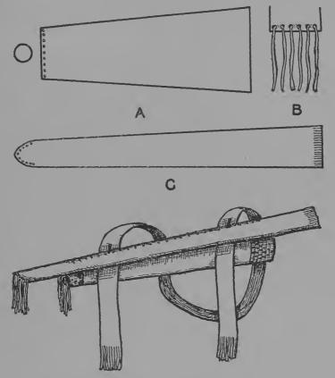
Fig. 92. (A) Quiver Pattern (B) Method of Making Fringe (C) Bow Case Pattern (D) Case and Quiver Complete
