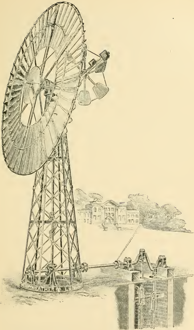
WIND WHEEL AND UPPER PART OF WELL.
