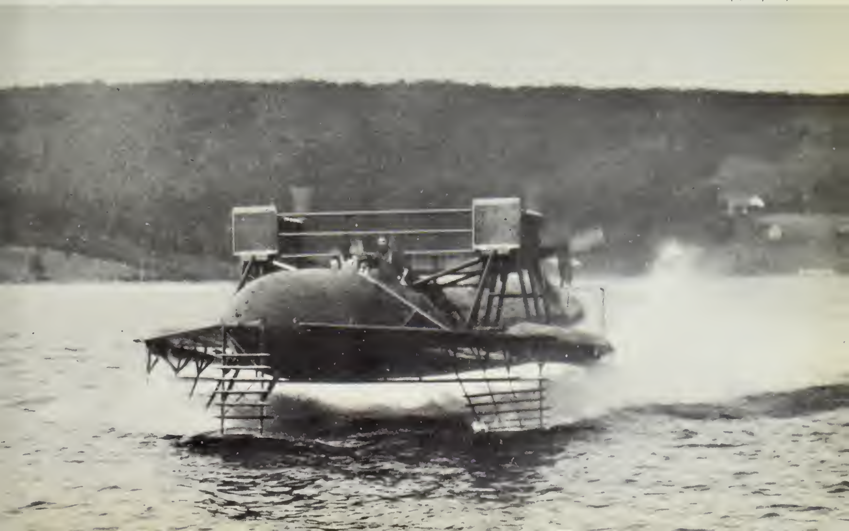
The experimental hydrofoil boat, Hydrodrome-4 , built by Alexander Graham Bell and F. W. "Casey" Baldwin, being tested at Baddeck, Nova Scotia, 9 September 1919. It reached a speed of 70.86 miles an hour.
