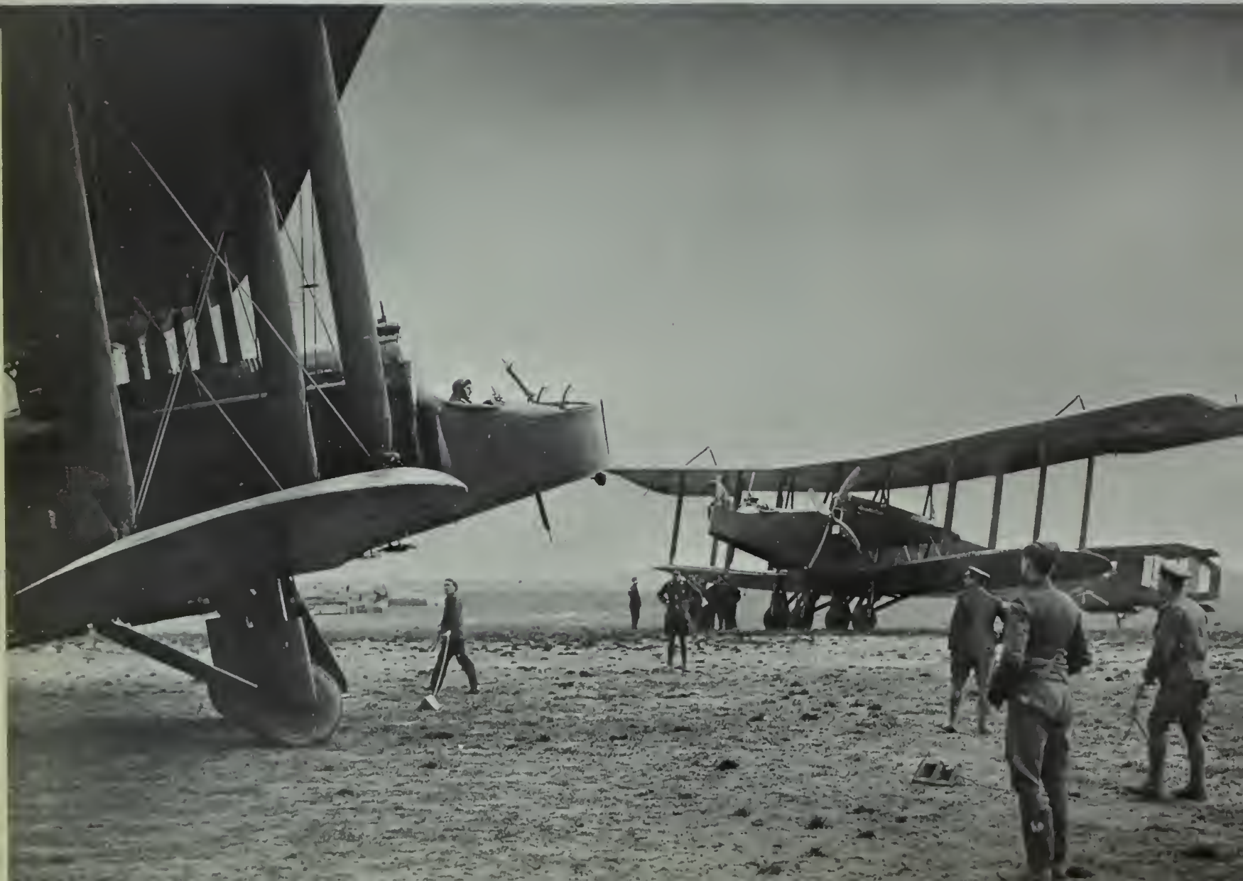
Below—Handley Page O/100 bombers on a Dunkirk-area field, April 1918. Many Canadians flew this big, night flying machine, which carried a bomb load of nearly 1800 pounds. (Courtesy Imperial War Museum)
