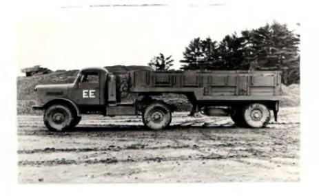
6 Ton Semi-Trailer -Body Code 2-H-1, for D.N.D. account, capacity 6 tons (12,000 lbs.).
