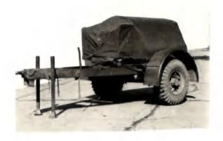
The function of this trailer is to supply 110 volt direct current for the operation of electrically driven tools and equipment in the R.E. 25 K.W. Machinery Lorry (described in Machinery Lorry Volume), and for the supply of power to one or more other Machinery Lorries. It also provides facilities for electric welding. for electric welding.
