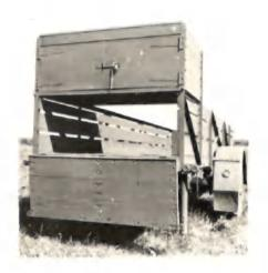
The trailer chassis of this vehicle was designed in three stages:-(a) Original design, with 9.00 x 16 tires, (b) Original design with revisions to chassis frame, and with 9.00 x 16 tires, (c) Same as 'b' but with 7.00 x 20 tires. In all three models, however, the body design was the same.
