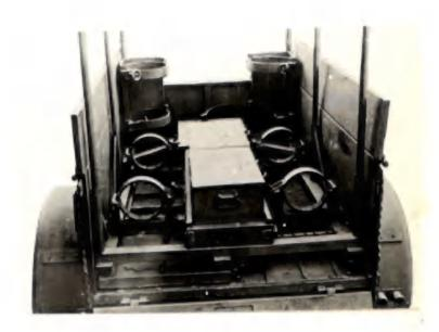
The function of this trailer is to provide facilities for oxy-acetylene welding and blacksmith work in the field.
