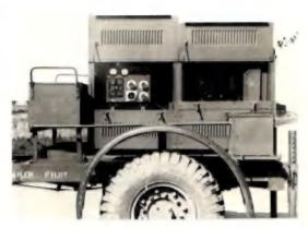
The function of this trailer is to supply 110-volt D.C. power for operation of Machinery Lorries in the field.
