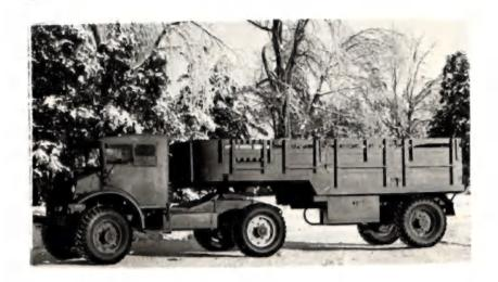
Semi-trailer body - Code 10-G-1, for British Ministry of Supply. Capacity- 6 long tons (13,400 lbs.)
