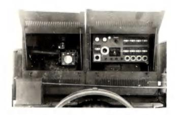
The function of this trailer is to supply 110-volt D.C. power for operation of Machinery Lorries in the field.
