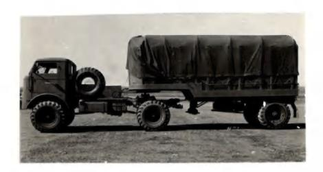
10 Ton Semi -Trailer equipped with Dolly for converting to full Trailer.
