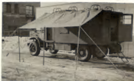
3-ton Wireless with Penthouse erected.
