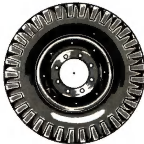
W.D. TIRE & WHEEL ASSY.—10.50-20 WT. 237 LBS.
