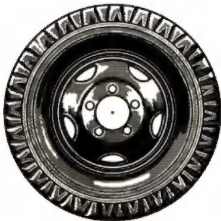
TIRE & WHEEL ASSY. 8.25-20 (COMMERCIAL) WT. 155 LBS.
