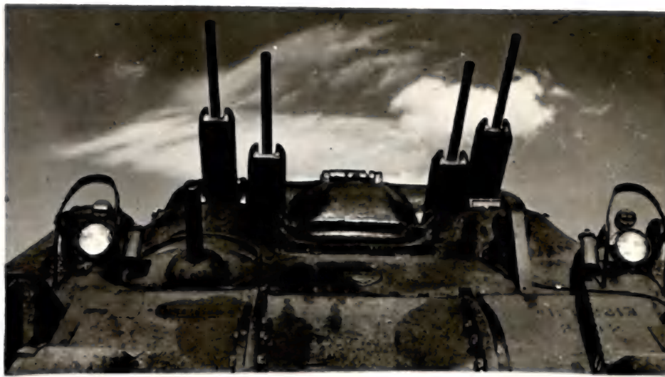
FRONT SILHOUETTE -Showing turret, gunner's hatch (closed) Polsten machine guns, bow gun, siren at left, M4A1 blackout and driving lights with weather seal plug housing shown on light guards (Plug to be used when lights are removed)
