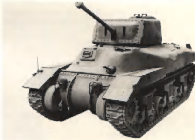
THREE-QUARTER LEFT FRONT VIEW - Showing tool box on left track guard, bow gun, 6-Pr. elevated, -Driver's indirect vision door and rotor in closed position and driver's and co-driver's periscopes.
