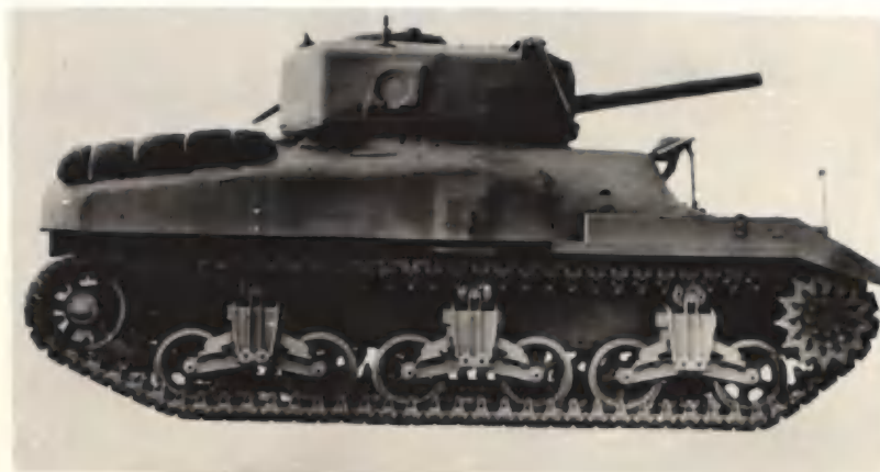
RIGHT SIDE VIEW -Showing driver's indirect vision door and rotor in the raised position, pistol port on side of cast armour turret and tool box on track guard.
