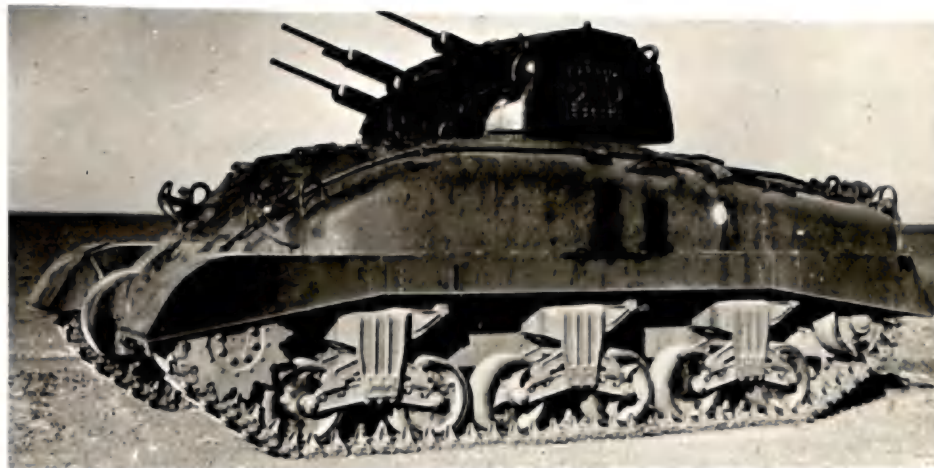
LEFT SIDE VIEW -Showing spare track shoes on side of cast armour turret and Polsten guns elevated. Ancillary equipment and towing cable in stowed position.
