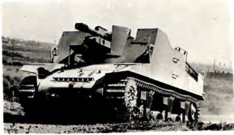
THREE-QUARTER LEFT FRONT VIEW -Action View. (Vehicle fitted with one- piece transmission and final drive, M4 type headlamps and stowage rack for spare track shoes.)
