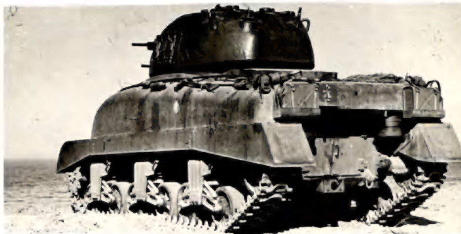
THREE-QUARTER LEFT REAR VIEW -Showing Base Aerials at rear of turret, water containers on rear of upper hull and air cleaners at rear of engine compartment.
