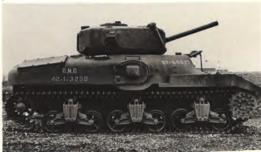
RIGHT SIDE VIEW -(early type)-Showing utility door in side of hull, pistol port and protectoscope on side of turret. (C.D.P. track and matching sprocket shown installed.)
