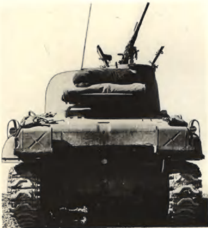
REAR VIEW-Showing general stowage arrangement at rear of turret and rear deck also .50 calibre anti-aircraft gun in position.
