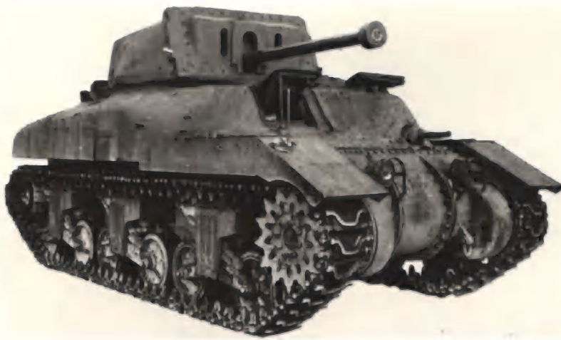
REE-QUARTER RIGHT FRONT VIEW -Showing driver's indirect vision door and rotor open. -driver's compartment hatch open, and rubber bushed T54E1 type track.
