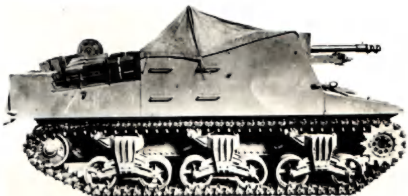
RIGHT SIDE-VIEW-Showing Bren guns and ammunition stowed on rear deck and canvas hood for crew compart- ment installed.
