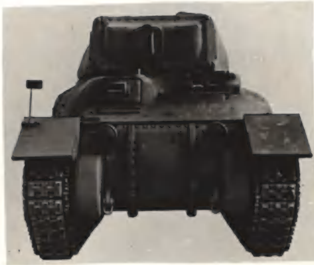
ONT VIEW -(early type hull)-Showing cupola type w gun mounting (Cupola later replaced by ball and socket type mounting)
