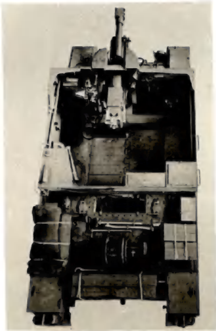
PLAN VIEW -Showing interior of crew compartment also tarpaulin, camouflage net, cable reel, Bren guns and ammunition and ancillary equipment stowed on rear deck. (Vehicle fitted with battery and auxiliary generator.)
