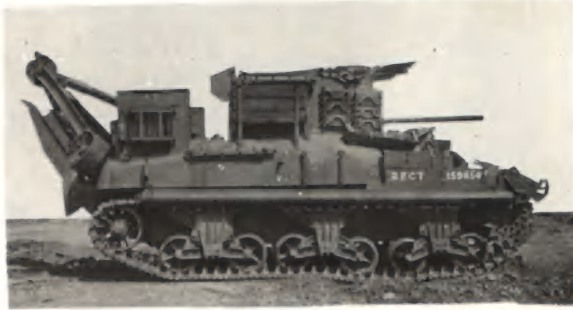
RAM II-MODIFIED AS ARMoured RECOVERY VEHICLE Used for recovery of bogged vehicles also to recover casualties out of range that are to be returned for repair. Vehicle shown is fully stowed.
